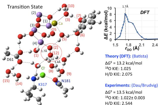
**Figure 1:** QM/MM model of the transition state for O-O bond formation at the OEC of PSII, based on the water nucleophilic attack (WNA) mechanism (left) and comparison to experimental kinetic data (right), including  $^{16}\text{O}/^{18}\text{O}$  and H/D kinetic isotope effects (KIE) and activation free energy values based on transition state theory.
