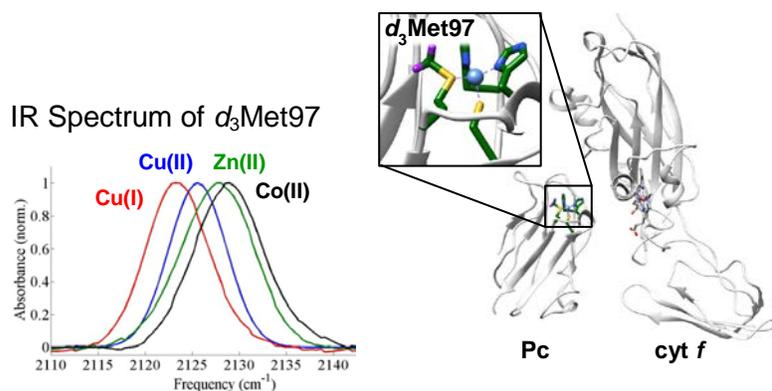
Figure 1. FT IR characterization of  $d_3$ Met97 of reduced, oxidized, and metal-substituted Pc.
