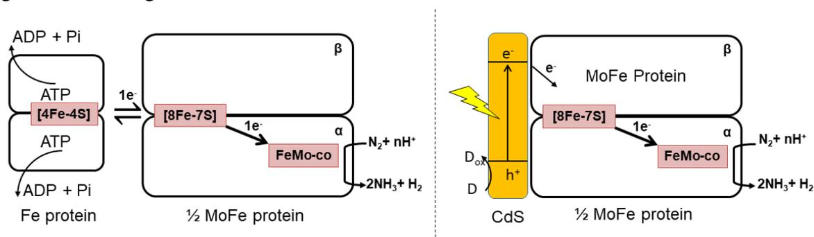
Figure 1. Left Panel: Schematic of nitrogenase proteins showing the delivery of electrons from the Fe protein to the MoFe protein driven by ATP hydrolysis. Right Panel: Schematic of the CdS nano-rod-MoFe protein biohybrid showing the light driven transfer of electrons into the MoFe protein protein to support  $N_2$  reduction.
