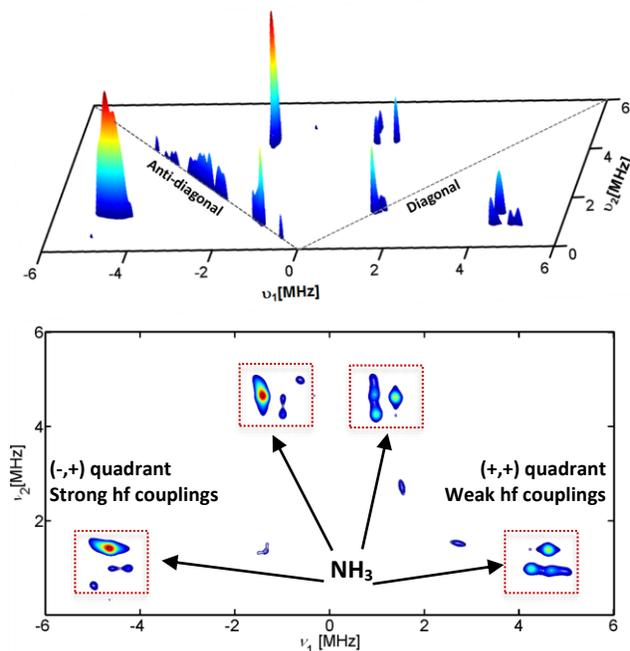
**Figure 1.** (A) Three- and (B) two-dimensional projections of the 2D  $^{14}N$  HYSCORE spectrum of the annealed  $S_2$  state of ammonia-treated PSII. The spectra display distinct cross-peaks that arise from the electron-nuclear hyperfine (hf) interactions of ammonia that is directly coordinated to the  $Mn_4Ca$ -oxo cluster in the annealed  $S_2$  state of ammonia-bound PSII.
