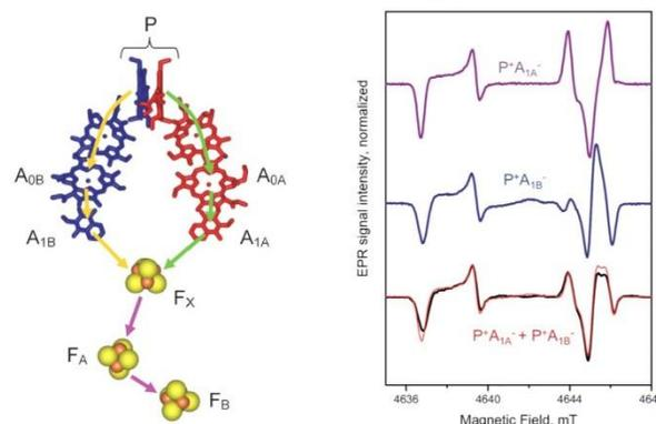
Figure 1. Schematic presentation of ET pathways in PSI and corresponding line-shapes of the spin-correlated high-frequency EPR
