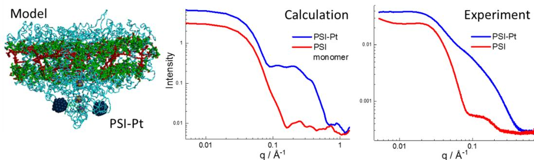
**Figure 1.** X-ray scattering characterization of PSI-Pt biohybrids. The left panel shows a model PSI-Pt structure composed a PSI monomer and two Pt<sub>55</sub> nanoparticles positioned at candidate docking sites. The middle panel shows calculated X-ray scattering for the PSI monomer and PSI-Pt model. Calculations using trimer assemblies are on-going. The right panel shows experimental scattering for PSI and the PSI-Pt biohybrid.
