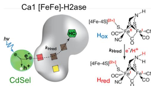
**Figure 2.** Photocatalytic CdSel:CaI complex and H-cluster reduction scheme for the initial proton-reduction step of  $H_2$  catalysis.
