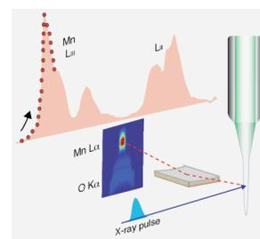
The reflection zone-plate emission spectrometer discriminates the weak Mn signal of PS II from the background of light atoms. PS II Sample is introduced with a liquid jet, and fs X-ray pulses from the XFEL enables the room temperature data collection possible.
