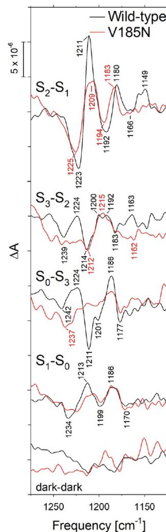
Figure 2.  $\text{D}_2^{16}\text{O}-\text{D}_2^{18}\text{O}$  double-difference spectra of wild-type (black) and D1-V185N (red) PSII core complexes in the D-O-D bending region.
