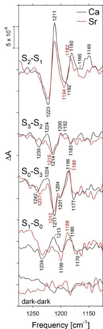
Figure 1.  $\text{D}_2^{16}\text{O}$ - $\text{D}_2^{18}\text{O}$  double-difference spectra of PSII core complexes containing  $\text{Ca}^{2+}$  (black) or  $\text{Sr}^{2+}$  (red) in the D-O-D bending region. From (2).
