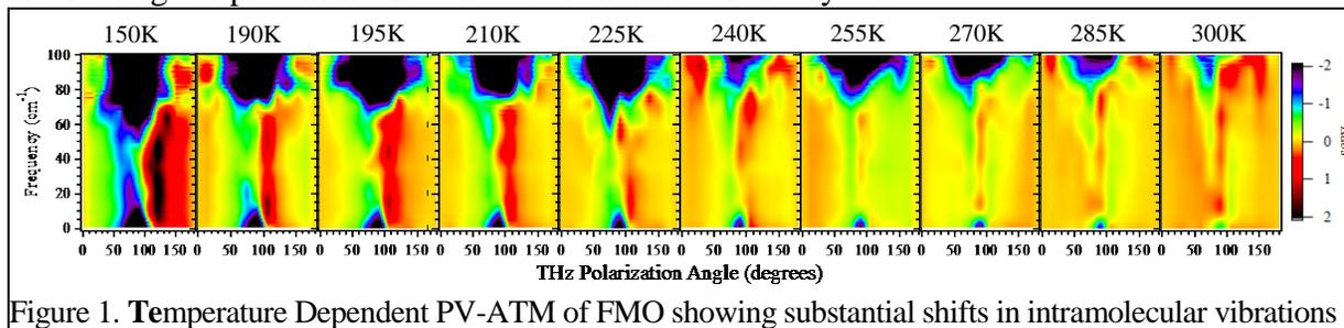
Figure 1. Temperature Dependent PV-ATM of FMO showing substantial shifts in intramolecular vibrations
