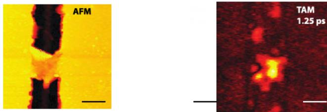
**Figure 1** Correlated AFM and TAM images for suspended graphene at two different delay times. Scale bars: 2  $\mu\text{m}$
