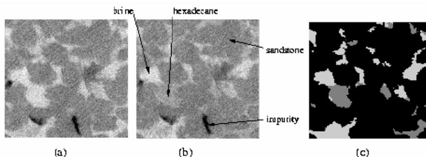
FIG. 1. A sub-region of the core image at a) water saturated and b) residual oil conditions. c) Phase identification results for b).
