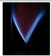
**Figure 3.** Photograph of the rod stabilized V-shaped flame impinging on a metal wall.
