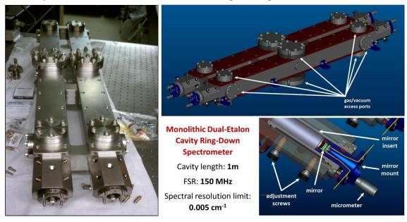
Figure 2: Photograph and schematic of DEFCOM spectrometer showing the two etalons bored out of a single piece of invar.
