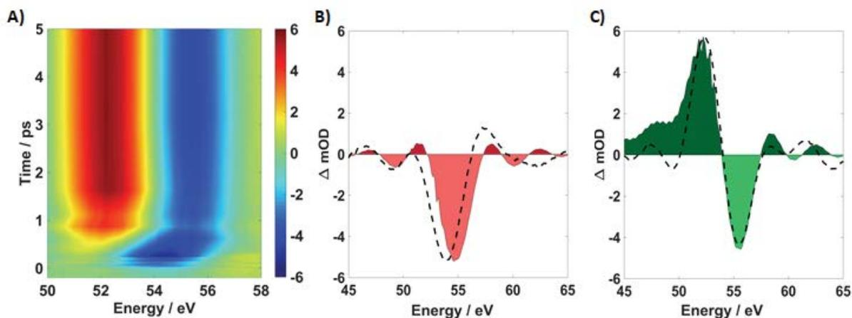
**Figure 2.** (A) Experimental contour plot showing the transient response at the Fe M-edge of photoexcited  $\text{Fe}_2\text{O}_3$  (B) Experimental (shaded red) and simulated (dashed line) initial photoexcited state of  $\text{Fe}_2\text{O}_3$  (C) Experimental (shaded green) and simulated (dashed line) final photoexcited state of  $\text{Fe}_2\text{O}_3$ .
