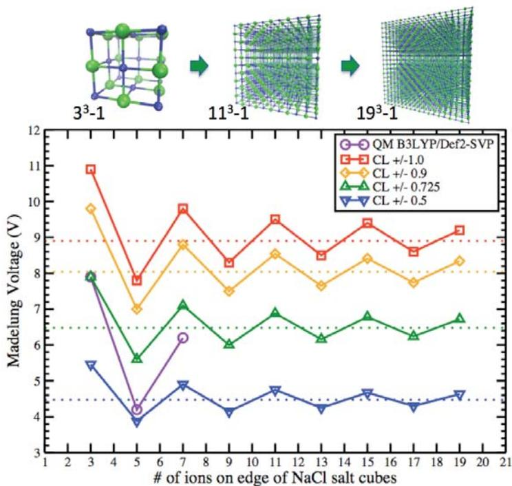
**Figure 2.** Classical (CL) and Quantum Mechanical (QM) Madelung voltage variations experienced by a central Cl<sup>-</sup> ion in NaCl clusters as a function of cluster size and ion charge. The QM voltages *cannot* be obtained by uniform scaling of the CL charges ( $|q| = 1.0, 0.9, 0.725, \text{ and } 0.5e$ ).
