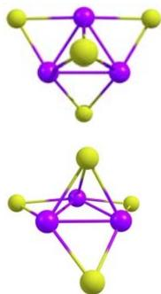
**Figure 3.** Top and side views of the optimized Mo<sub>3</sub>S<sub>4</sub><sup>-</sup> cluster structure.
