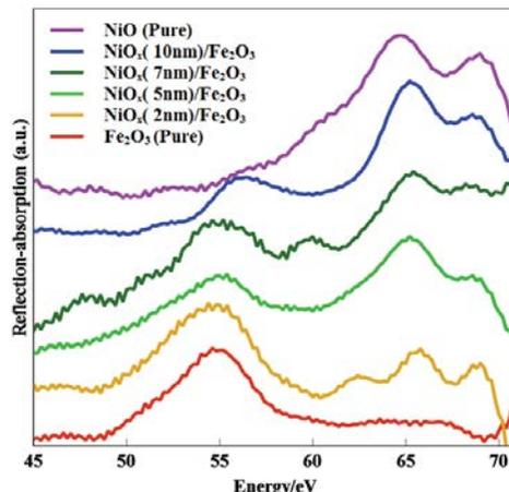
**Figure 3** Ground state RA spectra of several NiO<sub>x</sub>/Fe<sub>2</sub>O<sub>3</sub> heterojunctions compared with pure NiO (purple) and Fe<sub>2</sub>O<sub>3</sub> (red).
