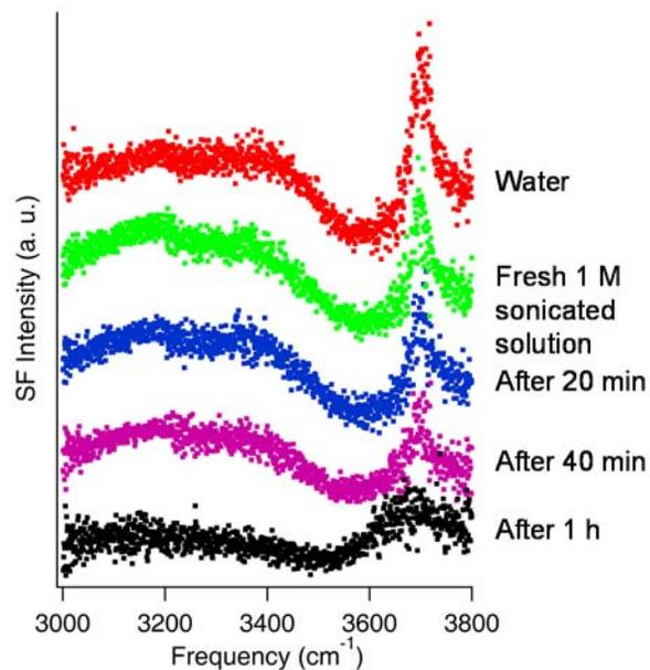
Figure 2. VSFG spectra of aqueous  $\text{FeCl}_3$  solution surfaces revealing time evolution of surface hydrolysis and water structures.
