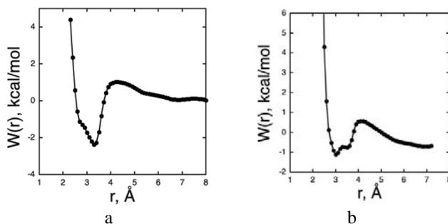
**Figures 5a and 5b.** Computed PMFs for  $\text{Li}^+[\text{BF}_4]/\text{Li}^+[\text{PF}_6]$  in EC at 330K.
