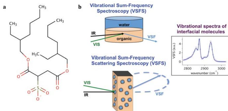
**Figure 1.** (a) The chemical structure of AOT. (b) A diagram of the planar and particle VSF experimental geometries, both involving an overlap of the incoming visible and IR beams at the planar interface (top) in a TIR geometry, or the center of a cuvette composed of a CaF<sub>2</sub> front window with a quartz back window and an optical path length of 200  $\mu$  m.
