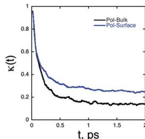
**Figure 3.** Computed  $\kappa(t)$  using the RF method for the NaCl ion pair in the bulk and at the Gibbs dividing surface.
