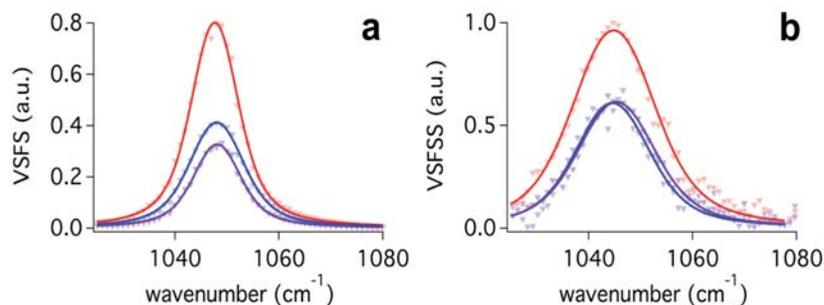
**Figure 2:** VSF SSP spectra of the S-O symmetric stretch of Na:AOT (blue), K:AOT (purple), and Mg:AOT (red) at the (a) planar isooctane/ D<sub>2</sub>O interface and (b) the CCl<sub>4</sub>/D<sub>2</sub>O reverse nanoemulsion interface. The spectral broadening is due to the difference in laser systems used.
