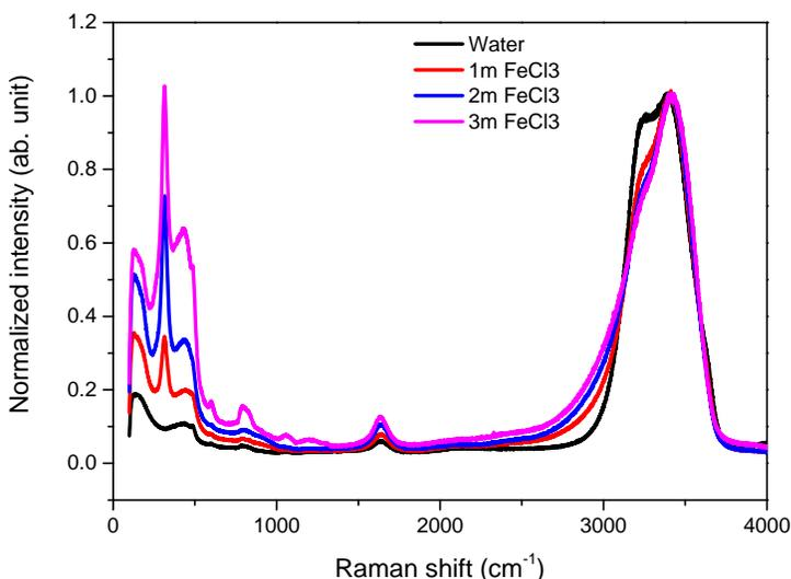
Figure 3. Unpolarized Raman spectra of bulk solutions revealing hydrogen bond network perturbation and iron speciation.
