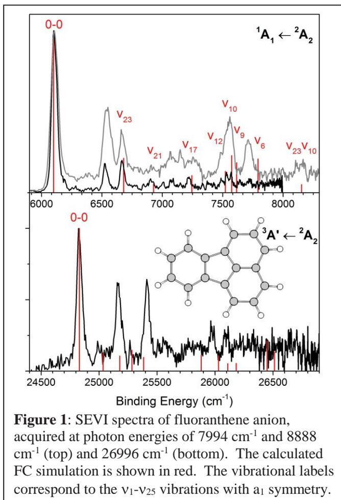
**Figure 1:** SEVI spectra of fluoranthene anion, acquired at photon energies of  $7994 \text{ cm}^{-1}$  and  $8888 \text{ cm}^{-1}$  (top) and  $26996 \text{ cm}^{-1}$  (bottom). The calculated FC simulation is shown in red. The vibrational labels correspond to the  $\nu_1$ - $\nu_{25}$  vibrations with  $a_1$  symmetry.
