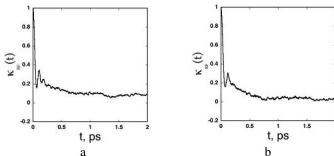
**Figures 6a and 6b.** Computed time-dependent transmission coefficients,  $\kappa(t)$ , for  $\text{Li}^+[\text{BF}_4]$ , (b) for  $\text{Li}^+[\text{PF}_6]$  in EC using the RF method.
