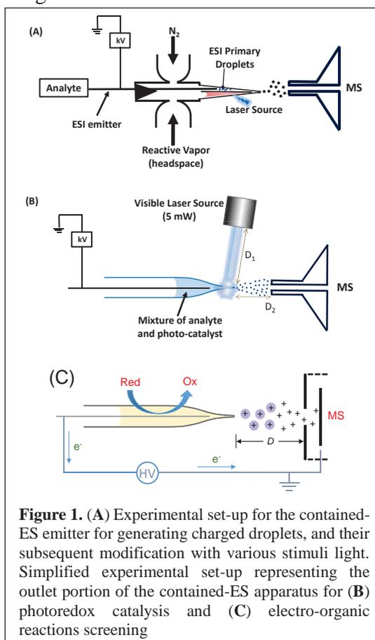
**Figure 1.** (A) Experimental set-up for the contained-ES emitter for generating charged droplets, and their subsequent modification with various stimuli light. Simplified experimental set-up representing the outlet portion of the contained-ES apparatus for (B) photoredox catalysis and (C) electro-organic reactions screening
