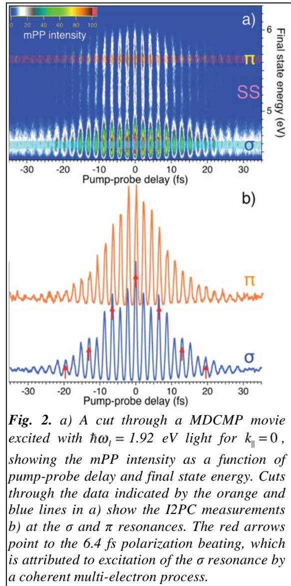
**Fig. 2.** a) A cut through a MDCMP movie excited with  $\hbar\omega_i = 1.92$  eV light for  $k_{\parallel} = 0$ , showing the mPP intensity as a function of pump-probe delay and final state energy. Cuts through the data indicated by the orange and blue lines in a) show the I2PC measurements b) at the  $\sigma$  and  $\pi$  resonances. The red arrows point to the 6.4 fs polarization beating, which is attributed to excitation of the  $\sigma$  resonance by a coherent multi-electron process.
