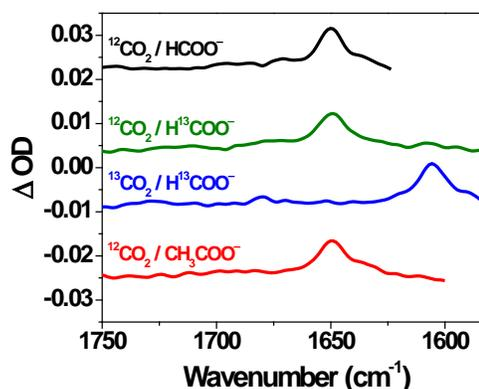
TRIR spectra recorded immediately after pulse radiolysis of  $\text{CD}_3\text{CN}$  containing various combinations of  $^{12}\text{CO}_2$ ,  $^{13}\text{CO}_2$ ,  $\text{HCO}_2^-$ ,  $\text{H}^{13}\text{CO}_2^-$ , and acetate.
