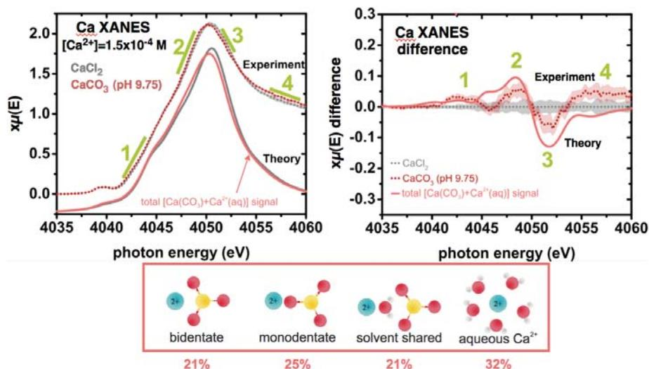
Figure 1. Experimental and theoretical (TDDFT-MD) XANES spectra for aqueous  $10^{-4} \text{ M Ca}^+$  (left) at pH 9.75. The difference spectra (right) represents the deviation due to the ion pair association with respect to that from the fully hydrated  $\text{Ca}^{2+}$ . The percentage distribution (lower) of three different ion pair species derived from the DFT potential of mean force. This distribution was used to calculate the theory XANES spectra.
