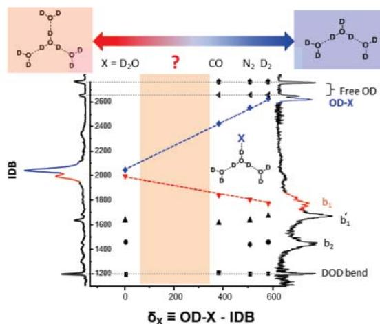
**Fig. 1.** The interpolation of band patterns from  $D^+(D_2O)_3$  (3D) to  $D^+(D_2O)_4$  (4D) using the OD-X band displacement relative to the location of the bound OD stretch fundamentals in 4D as an empirical index of intermediate distortion. The red “?” below the color bar emphasizes the need to add another tag species to quantify the band pattern in this range of the transformation from 3D to 4D.
