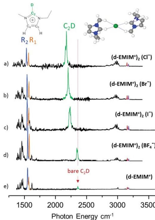
**Fig. 2.**  $N_2$ -tagged vibrational spectra of the cationic ternary clusters,  $(d\text{-EMIM}^+)_2X^-$ , where d-EMIM indicates selective deuteration at the  $C_{(2)}$  position. The green band near  $2300\text{ cm}^{-1}$  arises from the antisymmetric stretch of the  $C_{(2)}$ -D groups bound to the anions.
