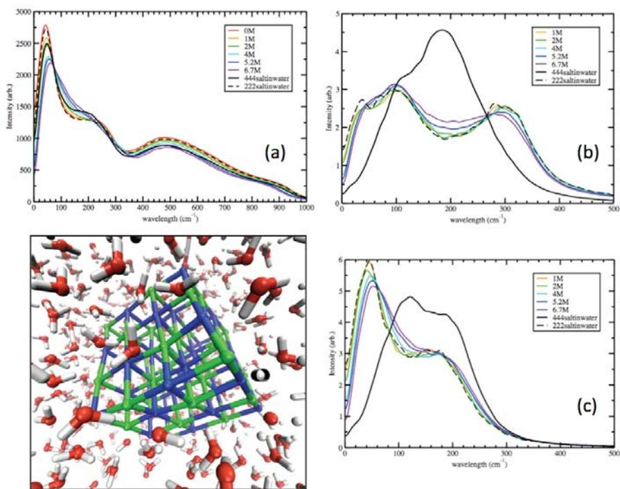
**Figure 3.** (a) Total vibrational power spectra for water and various concentrated NaCl electrolyte solutions including spectra for an unstable (dissociated)  $2^3$  NaCl crystal and stable (intact)  $4^3$  NaCl crystal (bottom left). (b) Sodium (Na) and (c) Chloride (Cl) spectra showing the vibrational signature corresponding to crystal formation.
