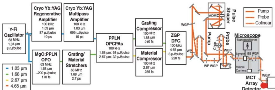
**Figure 2.** The general layout of 100 kHz mid-IR laser system and 2D IR microscope.
