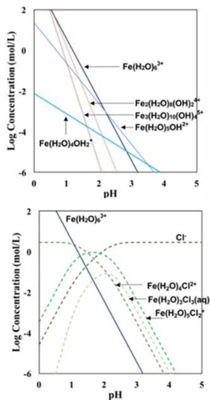
Figure 4. Calculated iron(III) speciation in bulk aqueous solution.
