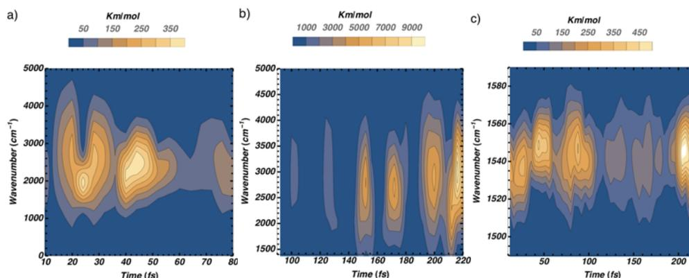
Figure 1. Transient vibrational spectra of (a) OH, (b) NH, and (c) backbone stretching modes following photoexcitation of the 2-(2'-hydroxyphenyl)-benzothiazole molecule from  $S_0$  to  $S_1$  state.
