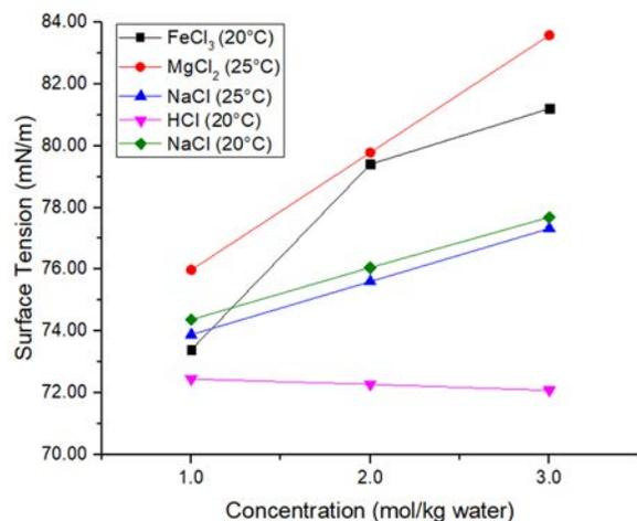
Figure 1. Surface tension of  $\text{FeCl}_3$  compared to other salts and HCl. Note that iron is an acid, yet it increases the surface tension of water similar to non-acids.
