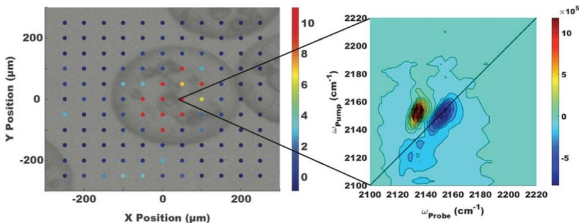
**Figure 3.** 2D IR microscopy image of a polystyrene bead with methyl thiocyanate in chloroform. The color bar represents the integrated intensity of the peak in the 2D IR spectrum associated with the  $\nu=1$  to  $\nu=2$  transition.
