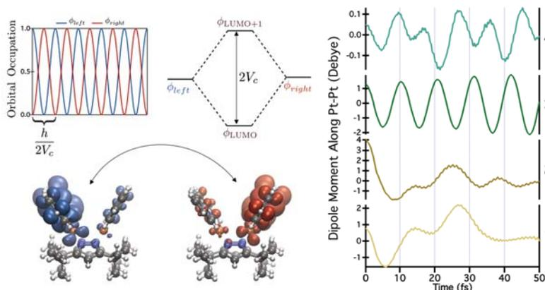
Figure 3. Left: Schematic of excited state coherence. The in-phase ( $\phi_{LUMO}$ ) and out-of-phase  $\phi_{LUMO+1}$  orbitals are formed from orbitals localized on either side of the system ( $\phi_{left}$  and  $\phi_{right}$ ). The coherent electron transfer can be analyzed in terms of the contribution of these localized orbitals to the time evolving density and dipole moment (Right).
