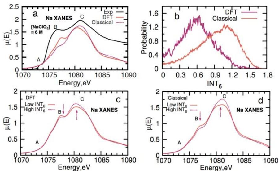
Figure 2. (a) Experimental XANES spectrum for Na<sup>+</sup> compared to TDDFT calculations for classical- and DFT-models that were generated from an ensemble average of 40 MD simulation snapshots, (b) the interstitial order parameter (INT6) for the 6<sup>th</sup> water hydrating Na<sup>+</sup>, (c,d) XANES spectra due to changes in the INT6 order parameter for DFT and classical models
