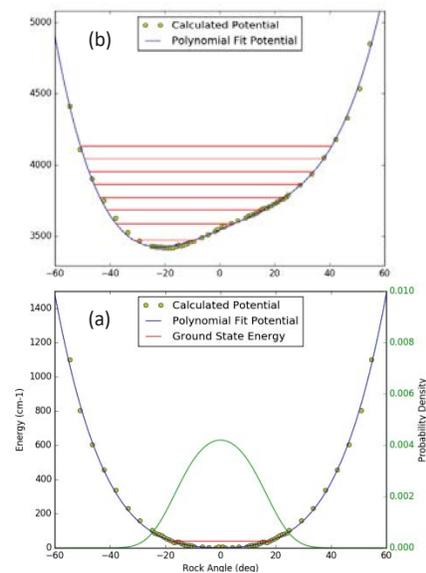
**Fig. 3.** Adiabatic potentials for water rock of  $NO_3^-(H_2O)$ . For (a)  $n = 0$  and (b)  $n = 1$  OH stretch adiabatic potentials. The wave function for the ground state rock level in  $n = 1$
