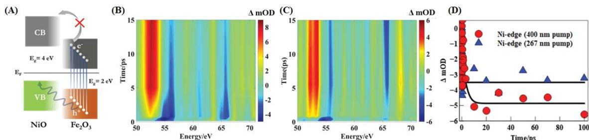
**Figure 4** (A) Band diagram of NiO/ Fe<sub>2</sub>O<sub>3</sub> heterojunction, showing the hole transfer across the interface. (B,C) Contour plots of the heterojunction photoexcited at 267 nm (B) and 400 nm (C), respectively. (D) Kinetic traces at the Ni edge pumped at 267 nm (blue markers) and 400 nm (red markers). Black solid lines show the fitted kinetics.
