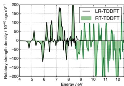
Figure 2. Computed electronic circular dichroism spectrum of  $\alpha$ -1,3-(R,R)-pinene. The vertical lines correspond to analogous LR-TDDFT results in cgs for the first 100 states. An artificial Lorentzian damping was applied to give the RT-TDDFT peaks a natural line width of 0.1 eV.
