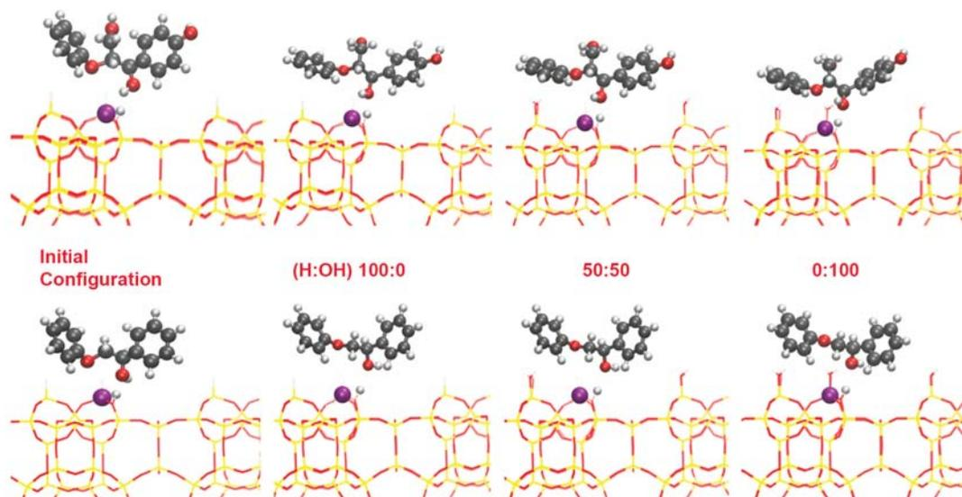
Figure 2. The effect of surface termination ( $-H$  vs  $-OH$ ) on the binding modes of model compounds with  $\beta$ -O-4 linkage (1-(4-hydroxyphenyl) 2-phenoxy-1,3-propanediol (HH, top) and 2-phenoxy-1-phenylethanol (PE, bottom)) on MWW nanosheet.
