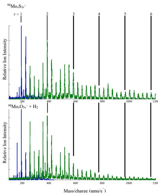
**Figure 1.** Top: Mass spectra of clusters generated from ablation of  $^{98}\text{MoS}_2$  powder, with  $\text{Mo}_x\text{S}_{3x}^-$  hypbersulfide clusters indicated. Bottom: cluster distribution following reactions with  $\text{H}_2$ . Blue and green traces are spectra obtained under low- and high-mass range settings on the mass spectrometer.
