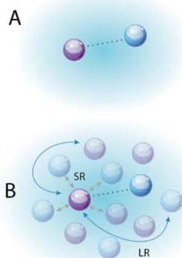
**Figure 2:** A schematic of a PMF of ion-pairing in the dilute limit (A) that was computed in **Figure 1**. (B) how the dilute limit PMF informs collective behavior. This will require the delicate interplay between the slowly varying long-range (LR) interaction and the complex short-range (SR) interaction.
