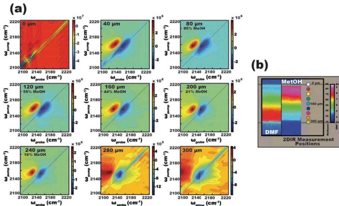
**Figure 1.** (a) 2D IR spectra collected across the microfluidic channel moving from 100% methanol to 100% dimethyl formamide by volume and (b) the IR chemical map images integrated from 3136 to 3189  $\text{cm}^{-1}$  for the solvent methanol and from 1720 to 1728  $\text{cm}^{-1}$  for the solvent DMF. The dots indicate the locations of 2D IR measurements across the channel.
