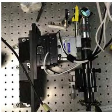
**Figure 1.** Photograph of microscope head to be integrated with a 100 kHz 2D IR spectrometer.
