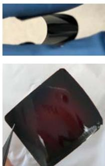
Figure 3. Pictures of heavily crosslinked s-PPBO-3K film
