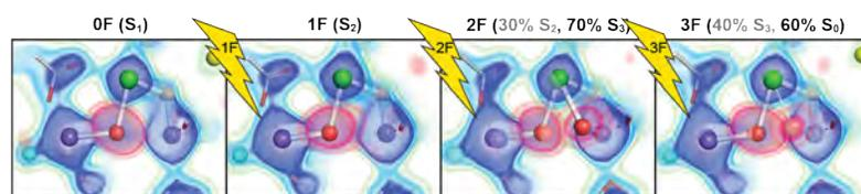
Electron densities for the S<sub>1</sub> through S<sub>0</sub> states, showing the new Ox in S<sub>3</sub>
