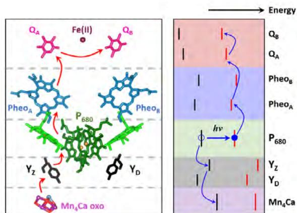
**Figure 1.** (a) The electron transfer cofactors of PSII as observed in the 1.9 Å resolution X-ray crystal structure<sup>1</sup> with the primary electron transfer pathway shown by red arrows. (b) An energy-level diagram illustrating the alignment of the HOMO and LUMO states of the cofactors. Blue arrows depict the electron and hole transport following charge separation at the primary donor, P<sub>680</sub>.
