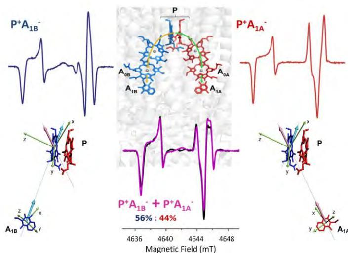
**Figure.** 130 GHz TR-EPR spectra of PSI complexes from fully deuterated cyanobacterium and schematic structure of ET pathways in PSI. SCRPs spectra and structure of RP for PSI were only A-branch is detectable (blue), only B-branch is detectable (red), both A- and B-branch are detectable (purple).
