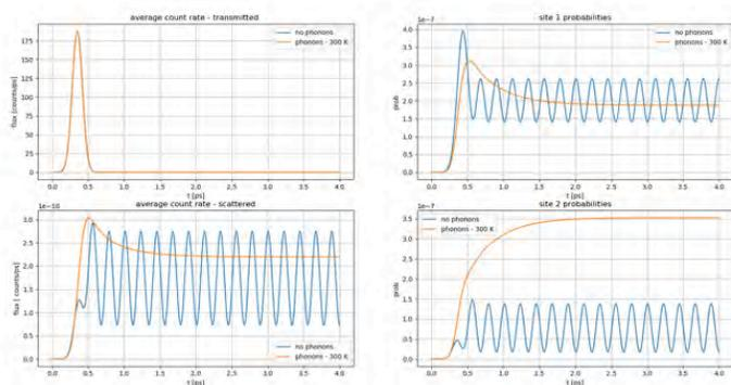
Figure 2. Average photon fluxes, i.e., counting rates, for transmitted and scattered photons (left panels) and corresponding excitation probabilities of two chromophores (right panels) resulting from incidence of a single photon on a light harvesting dimer as a function of time (ps) at T=300K. The effect of exciton-phonon coupling is to severely dampen the oscillations in both photon counting rates and chromophore excitation.
