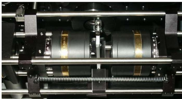
**Figure 1.** The Kerr-gate assembly consisting of Cassegrainian objectives, Kerr medium, polarizers and the injection mirror.
