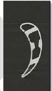
ORNL and Morris Technologies are using neutron scattering and imaging to improve understanding of the link between residual stress distortions and laser AM processing
