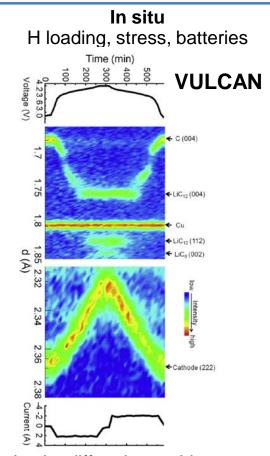
In situ diffraction on Li-excess layered compounds
