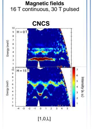
Spin excitations in Co<sub>3</sub>V<sub>2</sub>O<sub>8</sub>: 2D transverse field Ising model
