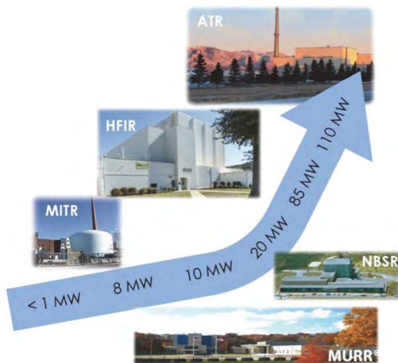
FIGURE 5b.1. Complementarity of research reactors based on the power output. The MITR, HFIR, and ATR reactors shown above the arrow are used for neutron irradiations to study materials degradation, while the MURR reactor provides irradiation to create special materials. The larger reactors also provide non-destructive characterization.
