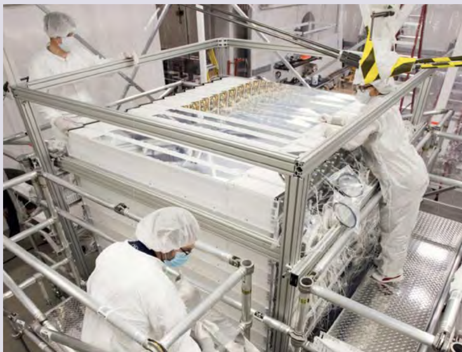
FIGURE B. Assembly of the segmented PROSPECT detector at the Yale Wright Laboratory prior to its shipment to ORNL/HFIR
