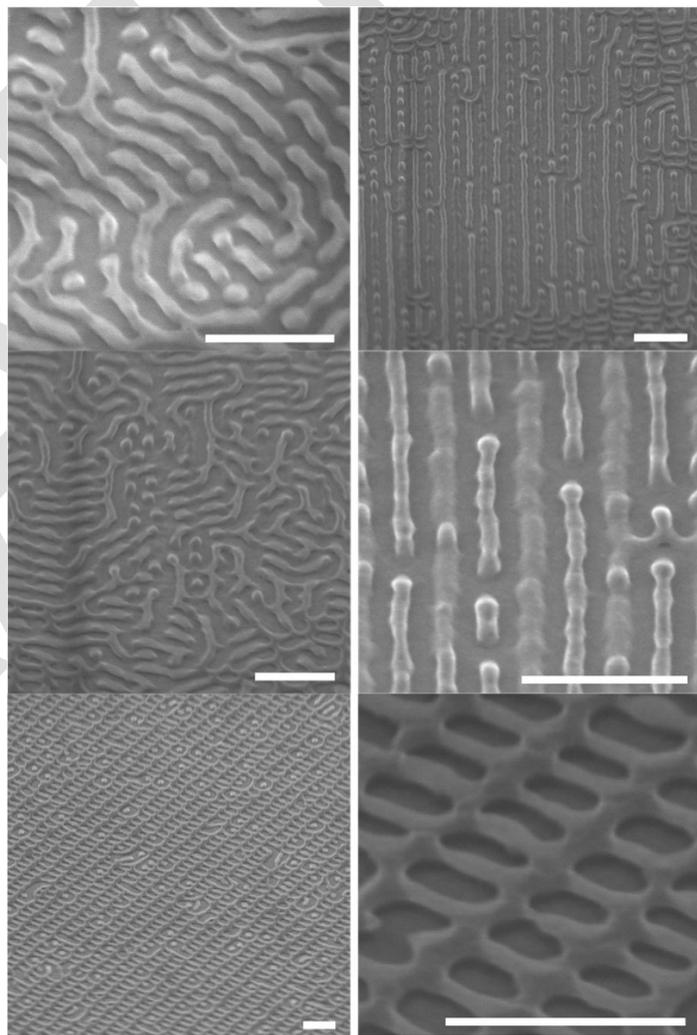
**Scanning-electron microscopy images of new nanostructures discovered using AI to lead autonomous experiments. All scale bars represent 200 nm. Image by the Center for Functional Nanomaterials (CFN).**
