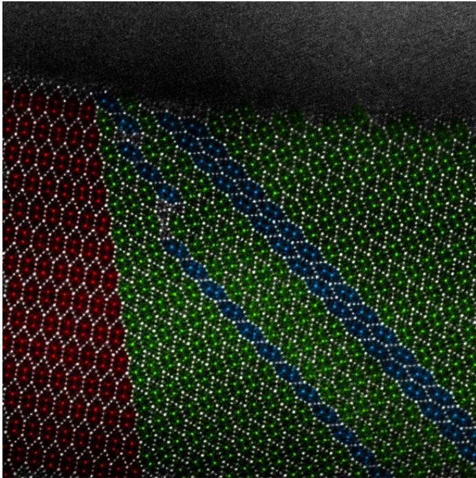
Atomic-resolution image of an  $\text{Al}_{94}\text{Mn}_2\text{Be}_2\text{Cu}_2$  alloy exhibiting superplastic behavior. False color was added to highlight the three primary twin orientations within the field of view (20 nm). Image by Jim Ciston, Colin Ophus, and Boštjan Markoli.
