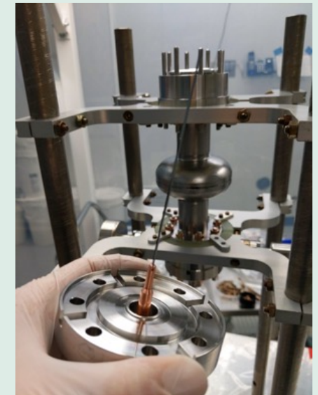
Integration of high-quality cavities with qubits
