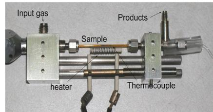
In a micro-reactor the catalyst can be exposed to different pressures and temperatures
