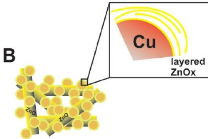
Active phase of the catalyst has an inverse oxide/metal configuration
