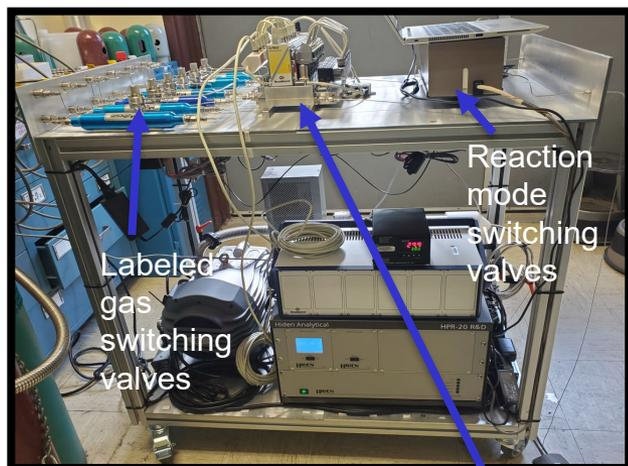
Mass flow controllers and shutoff valves for handling gases
