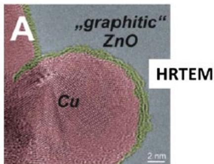
TEM studies for Cu/ZnO powder catalysts indicate that the active phase of the system consists of copper particles decorated with ZnO<sub>x</sub> clusters
