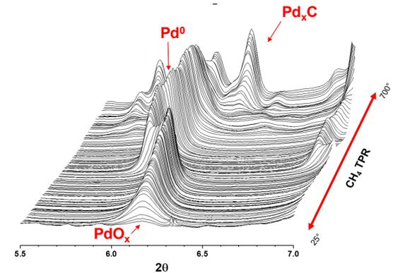
Evolution of active phase as a function of pressure and temperature
