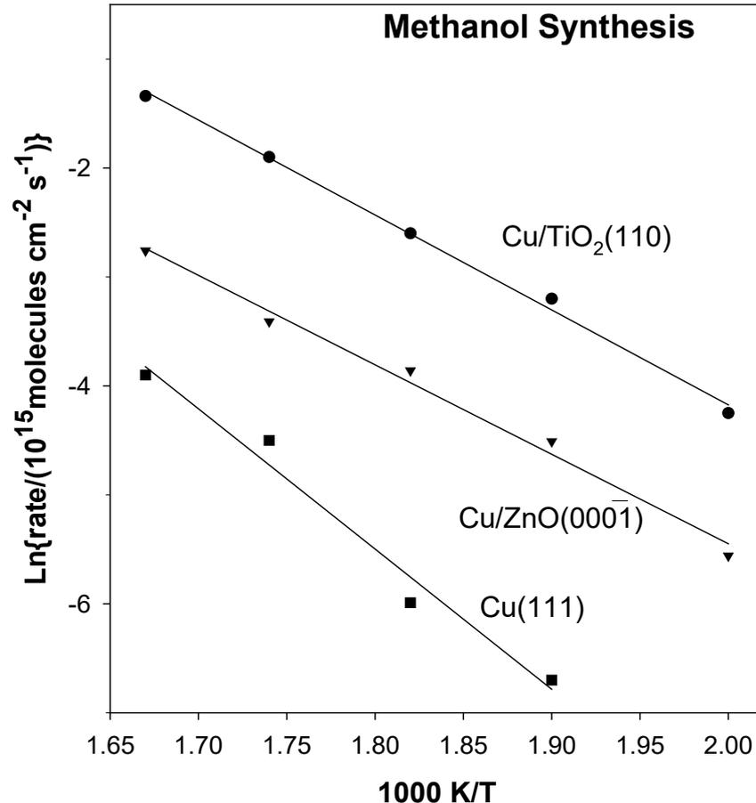
**Cu nanoparticles are more active than Cu(111) for the synthesis of methanol from CO<sub>2</sub> hydrogenation.**
