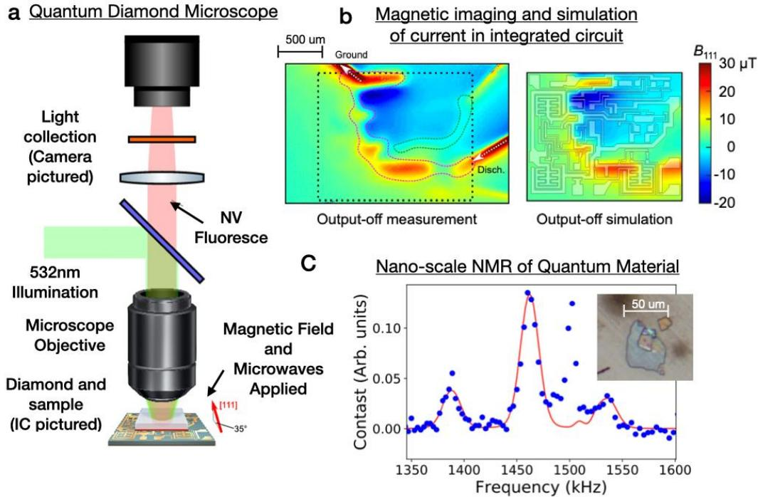
(a) Cartoon of Quantum Diamond Microscope experimental implementation at CINT. (b) Widefield quantum-sensed magnetic fields from integrated circuit and complete modeling of device.[2] (c) NMR spectrum for  $^{11}\text{B}$  in hBN as detected by nitrogen vacancy ensembles. (inset) 100nm thick hBN flake on nitrogen vacancy rich diamond. [3]
