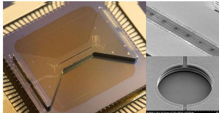
*Surface ion traps offer a scalable quantum computing platform with unparalleled fidelities. Recent advances include the integration of photonics for individual addressing and readout.*
