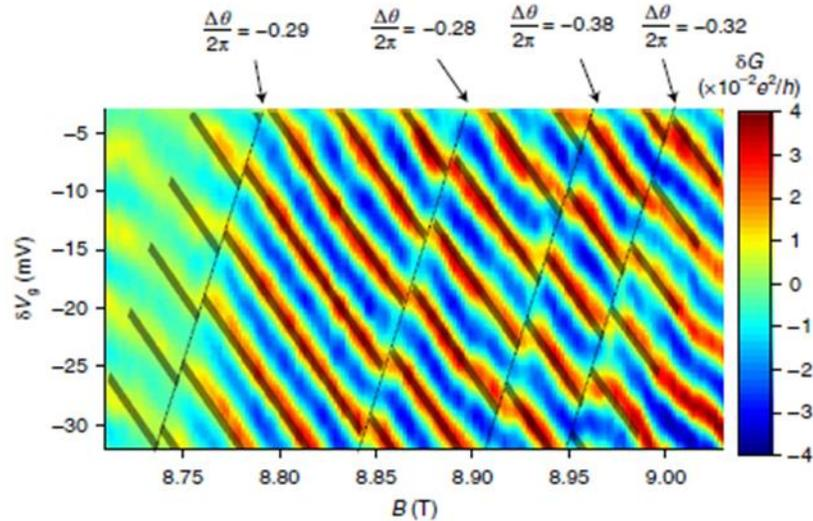
Map of the conductance (color scale) versus magnetic field ( $B$ ) and gate voltage in a 2D electronic device. Each dashed line denotes a jump in the phase of the quantum-mechanical wave of the system, corresponding to a rotation of a fraction ( $1/3$ ) of  $2\pi$ . This fractional rotation is the smoking gun for the presence of exotic particle-like objects called anyons.
