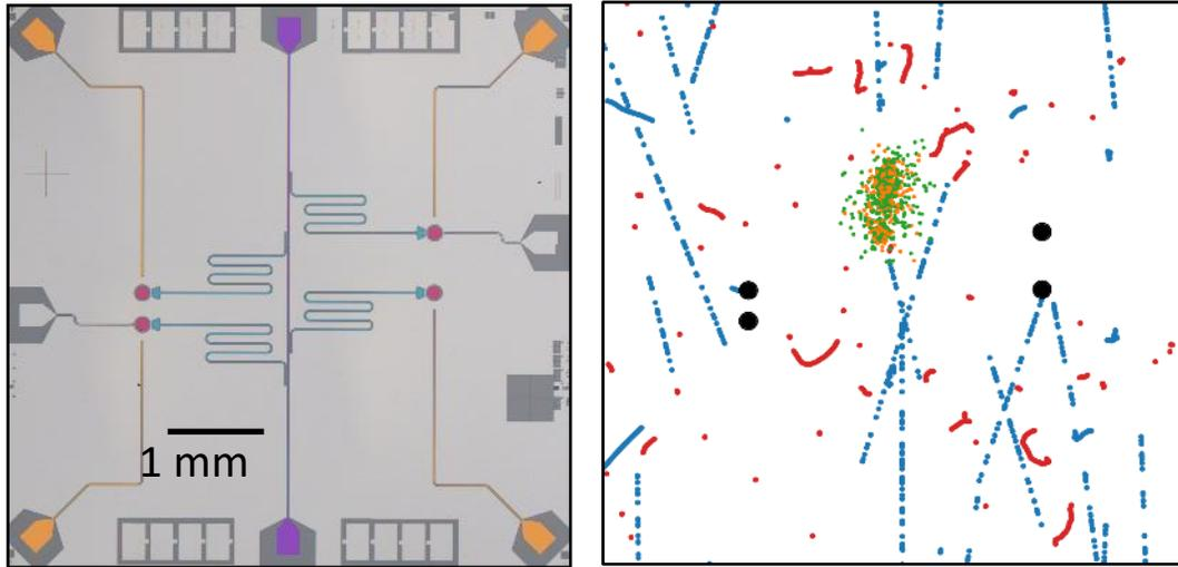
LEFT: Superconducting multiqubit (red circles) chip used to probe correlated errors.
