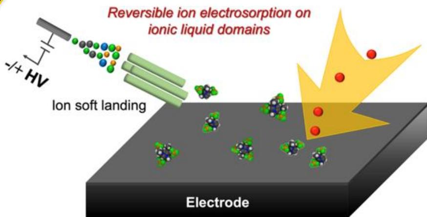
Dissolved ILCs are ionized by electrospray ionization and then deposited onto the electrode surfaces. Once adsorbed, the ILCs reduce the amount of energy needed for other ions from solution to adsorb and separate on the electrode.
