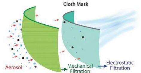
**Mask fabrics combining mechanical and electrostatic filtration**, such as a layer of high thread count cotton followed by a layer of silk, performed best. (CNM, Image courtesy of American Chemical Society)
