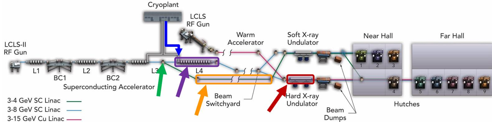
1. Add 20 additional cryomodules (L4 linac) to increase the LCLS-II accelerator energy to 8 GeV.
