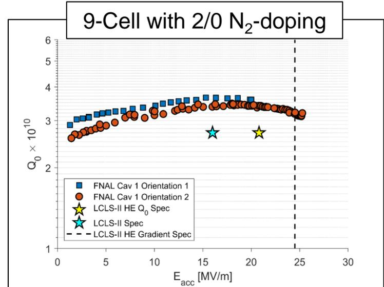
2/0 cavity processing method can produce 9-cells that meet LCLS-II HE spec!
