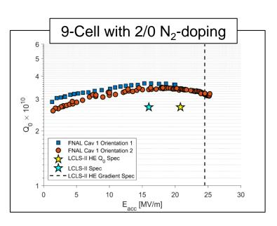
2/0 cavity processing method can produce <u>9-cells</u> that meet LCLS-II HE spec!
