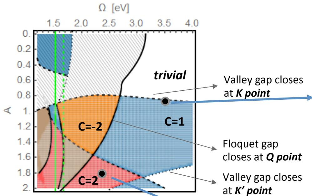
Tuning the band structure of a 2D material with light to create new topological phases and edge states.
