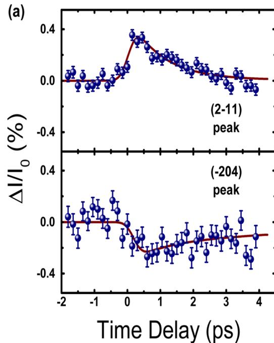
**Time resolved XRD for photoinduced superconductivity (Cavalleri et al)**
