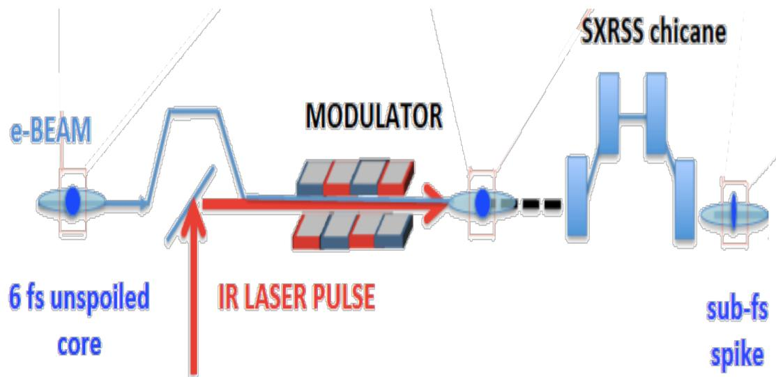
**Production of sub-femtosecond X-ray pulses**
