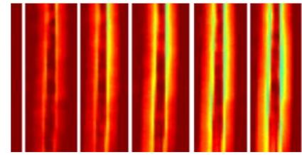
Neutron imaging of batteries in operation
