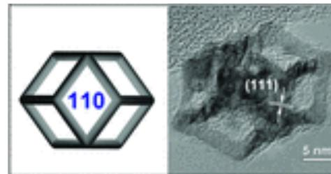
**PtNi<sub>3</sub> nanoframe with very high ORR electrocatalytic activity**
