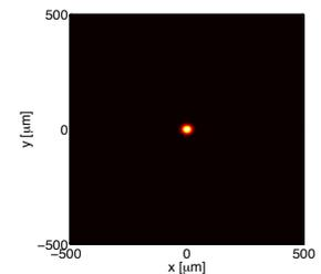
“DLSBs” have circulating electron beams small enough that the spot size and divergence of emitted x-rays is dominated by the fundamental diffraction of light, and not by the electron beam
