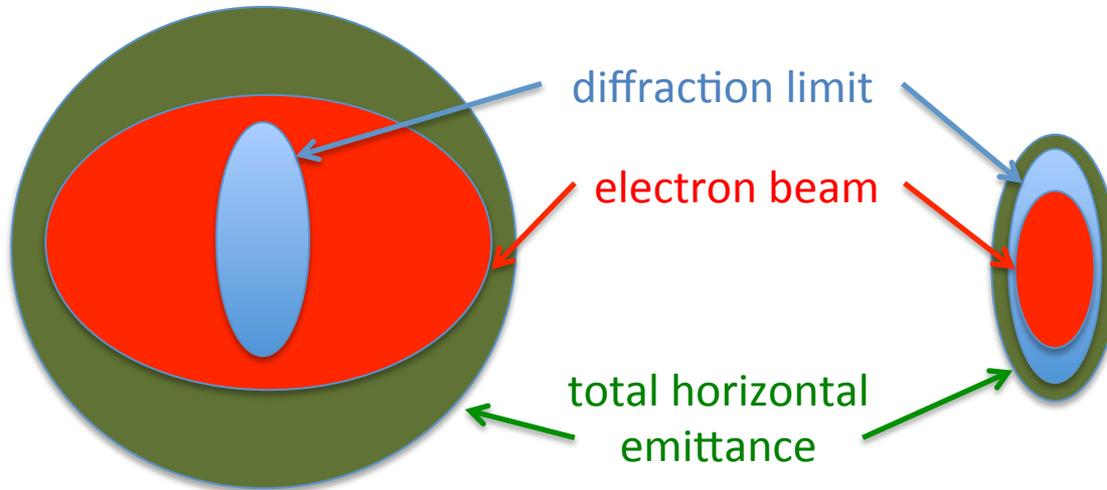
Multi-bend achromat magnets will allow us to get to the diffraction limit
