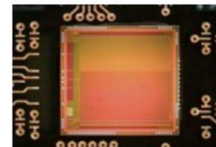
5  $\mu\text{m}$  CMOS detector- Denes
