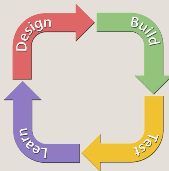
**Fig. 9. Design-Build-Test-Learn Cycle.** An iterative design strategy is based on the cyclic process of developing an initial design or prototype, testing that prototype, analyzing its performance against specific metrics, learning what worked and what did not work, designing a new prototype based on what was learned, and completing the cycle again. The goal is to improve design or prototype quality and functionality.
