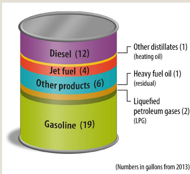
**Fig. 11. Products Made from a Barrel of Crude Oil.** A 42-gallon (U.S.) barrel of crude oil yields about 45 gallons of petroleum products. Falling under the “other products” category are petrochemicals including naphtha, ethane, ethylene, and other oils. [Image courtesy U.S. Energy Information Administration]
