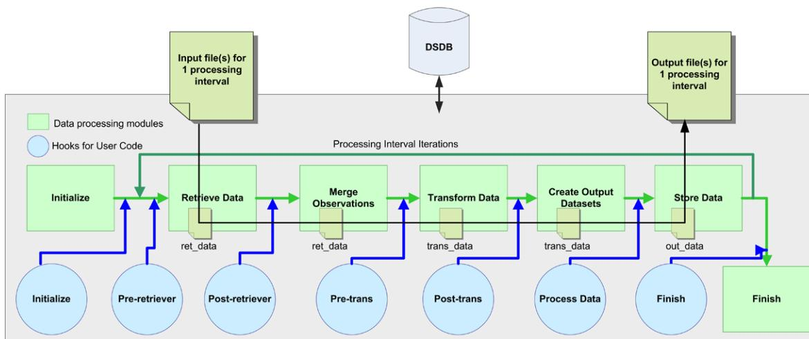
**Fig. D5-1. ARM ADI Workflow and Framework Hooks.** [Gaustad, K., et al. 2014. "A Scientific Data Processing Framework for Time Series Net CDF Data," *Environmental Modelling and Software* **60**, 241–49. Reprinted by permission of Elsevier Ltd.]
