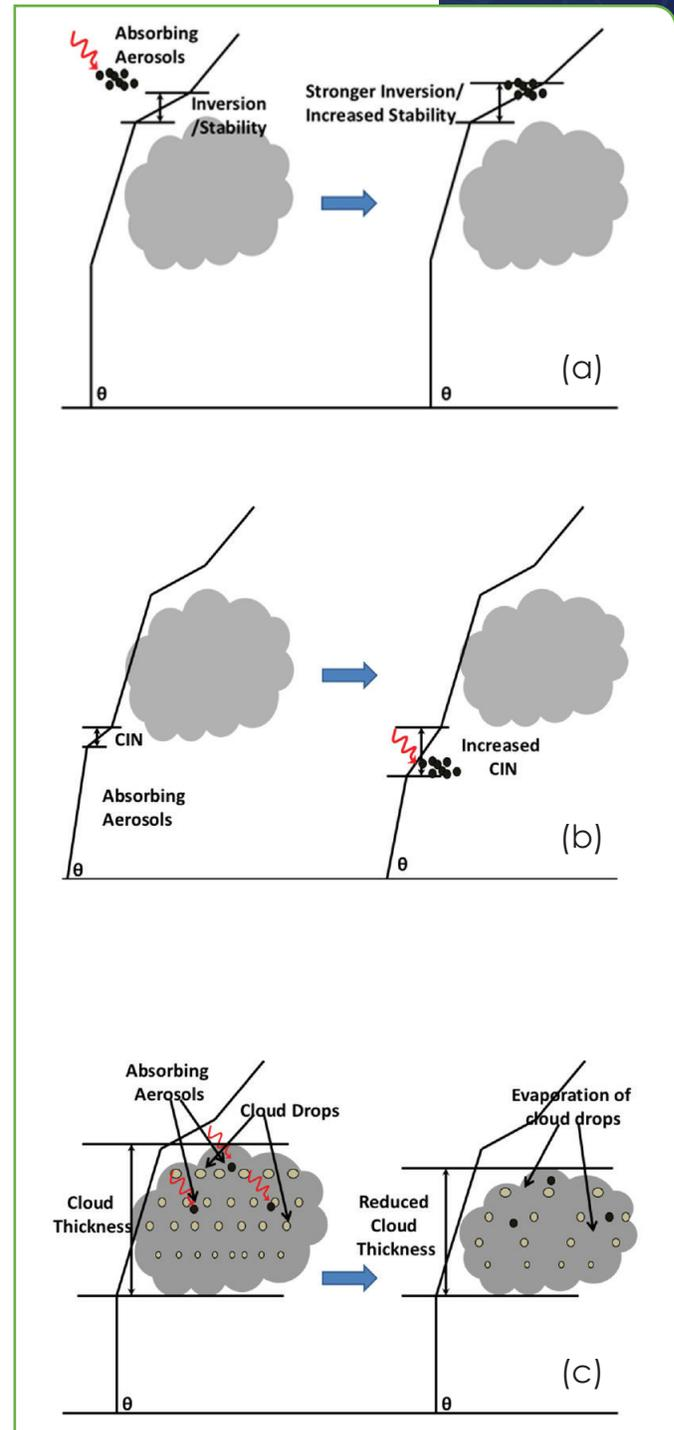
Hypothesized impact of absorbing aerosols on (a) boundary-layer inversion, (b) convective inhibition, and (c) cloud size and drops is shown here. CIN, convective inhibition, is a quantitative measure of the inhibition of convective activity; lower CIN implies lower stability.
