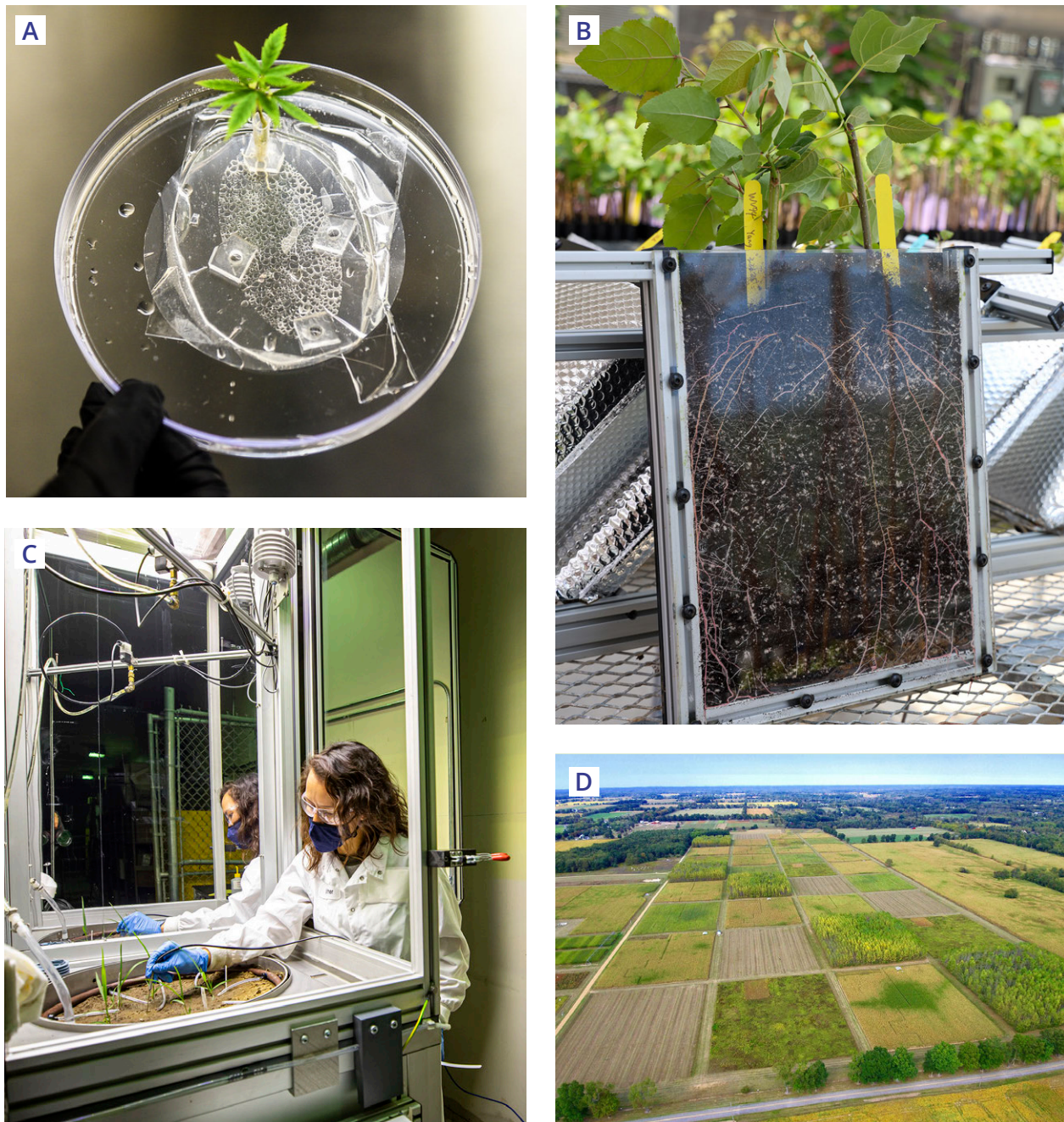
Fig. 4.1. Platforms for Testing Microbiome Engineering Span Micro- to Macroscales. (A) Microfluidic devices such as the rhizosphere-on-a-chip platform (RhizoChip) provide a microscale soil environment that retains the physical structure of natural soils and can be used to map the molecular environment of roots. [Courtesy Environmental Molecular Sciences Laboratory] (B) A Rhizobox soil observation system enables visualization of root growth and interactions with rhizosphere soil. [Courtesy Oak Ridge National Laboratory] (C) A scientist inspects plants growing inside an EcoPOD. EcoPODs are enclosed environments enabling intensive monitoring and manipulation of replicated plant–soil–microbe–atmosphere interactions over the complete plant life cycle. [Courtesy Lawrence Berkeley National Laboratory] (D) An aerial view of different treatments in a field research site at the Great Lakes Bioenergy Research Center and the Kellogg Biological Station’s Long Term Ecological Research Cellulosic Biofuels Research Experiment. This long-term study examines the impact of different cropping systems on ecosystem services related to biofuel crops. [Courtesy Kevin Kahmark, Michigan State University]
