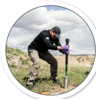
Molecular Observation Network (MONet). A MONet researcher extracts a core of soil to analyze in the lab. [Courtesy Andrea Starr, Pacific Northwest National Laboratory]
