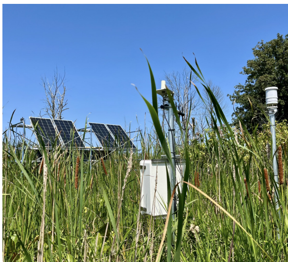
Fig. 2.3. Gathering Continuous Ecological Data Demands Energy Infrastructure and Data Logging. Solar panels (left) supply power to sensors and dataloggers at one of the COMPASS-FME wetland research sites in Ohio. The pole (right) includes sensors for photosynthetically active radiation, temperature, relative humidity, wind, and precipitation. The datalogger in the white box (center) collects these data as well as data from unseen belowground and aboveground sensors such as tree sap, soil moisture, temperature, and other environmental conditions. [Courtesy Nick Ward, Pacific Northwest National Laboratory]
