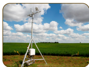
Eddy covariance system deployed at the Atmospheric Radiation Measurement (ARM) Central Facility and operated under the ARM Carbon Project umbrella at Lawrence Berkeley National Laboratory. [Courtesy Lawrence Berkeley National Laboratory]
