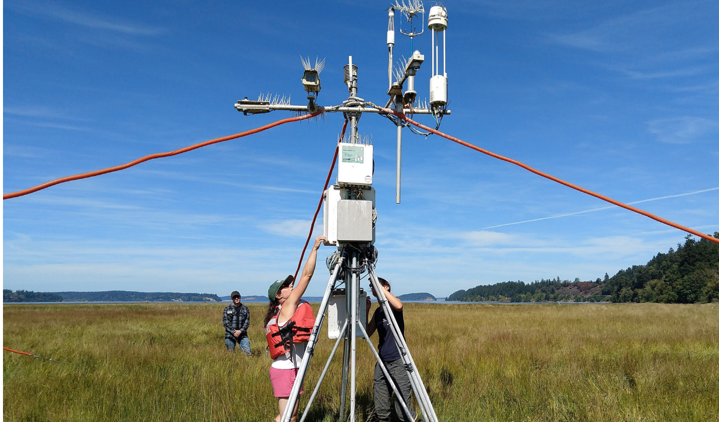
Researchers inspect an eddy covariance flux tower at Billy Frank Jr. Nisqually National Wildlife Refuge. [Courtesy AmeriFlux]
