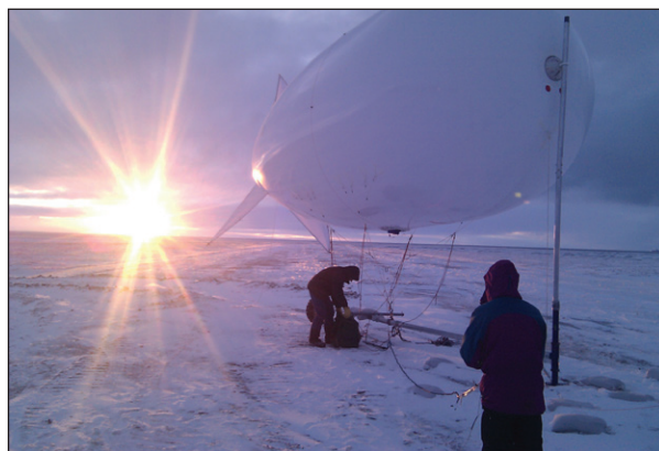
Fig. 9. Tethersonde Test Flight. Tethersondes, like this one, are used to collect atmospheric measurements at the Atmospheric Radiation Measurement (ARM) User Facility’s mobile observatory at Oliktok Point, Alaska. [Courtesy ARM User Facility]
