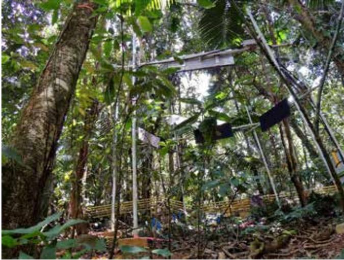
**Figure C.3.1.** Four rings at the Oak Ridge National Laboratory FACE experiment.
