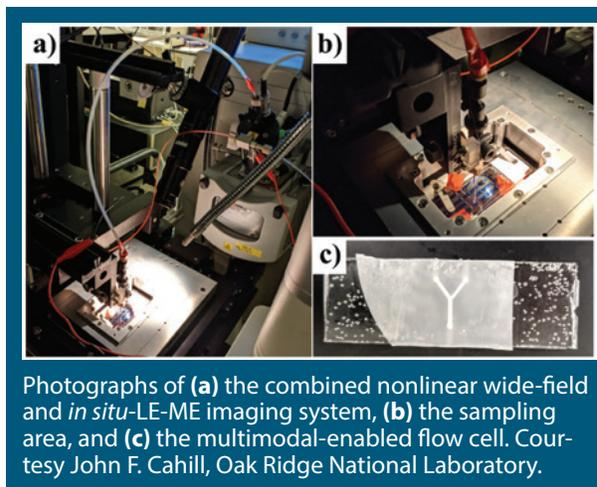
Photographs of (a) the combined nonlinear wide-field and *in situ*-LE-MS imaging system, (b) the sampling area, and (c) the multimodal-enabled flow cell. Courtesy John F. Cahill, Oak Ridge National Laboratory.
