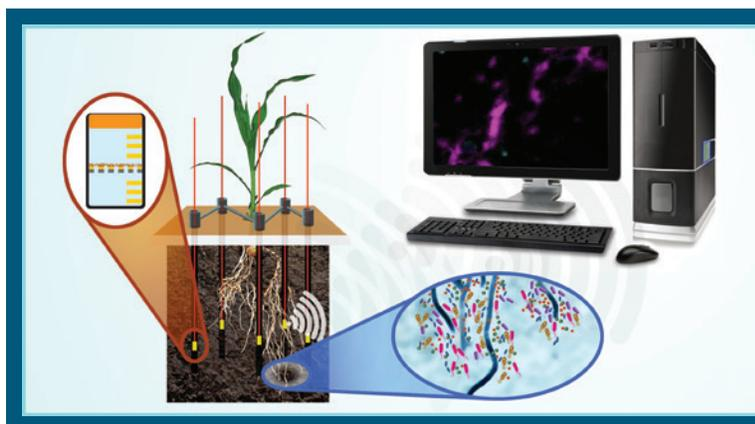
4DMAPS aptasensors are attached to moveable rods in shafts around a plant root. The sensors report wirelessly on the concentration of a specific molecular component to a receiver. The collected data are integrated to show where around the plant root a particular chemical compound is located and how this changes with time. Courtesy Ames Laboratory.
