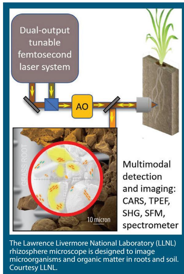
optimized the AO testbed optical system and carried out low-order AO corrections on synthetic soil samples, with the Strehl ratio tripled. Next steps are to perform high-order AO corrections and then integrate the AO system with the multimodal, multiphoton microscope.
