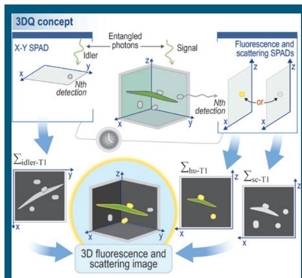
**Quantum-Enabled Techniques.** BSSD researchers are developing quantum imaging modalities, such as the three-dimensional quantum microscope illustrated here, which will use entangled photon pairs to obtain information beyond standard fluorescence or scattering measurements. Courtesy Lawrence Livermore National Laboratory.
