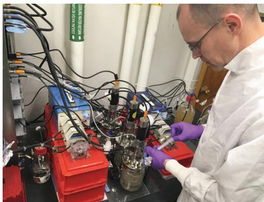
**Consolidated Bio-processing (CBP).** CBI researcher Evert Holwerda uses a microbial bioreactor with precise measurement tools to optimize biomass deconstruction and conversion to advanced biofuels and bioproducts. Ultimately, this CBP approach will eliminate the need for added enzymes and pre-treatment. [Dartmouth College]
