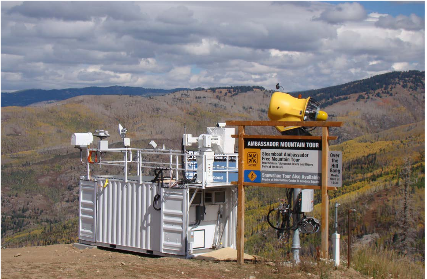
The AMF2 obtained data about liquid and mixed-phase clouds during the Storm Peak Laboratory Cloud Property Validation Experiment (STORMVEX) field campaign around Steamboat Springs, Colorado. AMF2 instruments were used in conjunction with Storm Peak Laboratory, a cloud and aerosol research facility operated by the Desert Research Institute.
