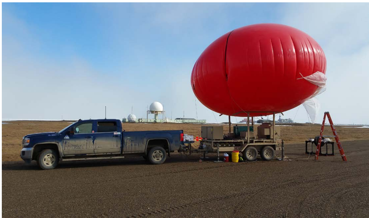
The tethered balloon system (TBS) operates up to 1.5 kilometers (0.93 miles) above Oliktok Point and AMF3 to collect atmospheric data such as temperature, humidity, and aerosols. Combining TBS measurements with deployments can provide a unique opportunity to collect valuable measurements of spatial context to vertically profiling AMF instruments.
