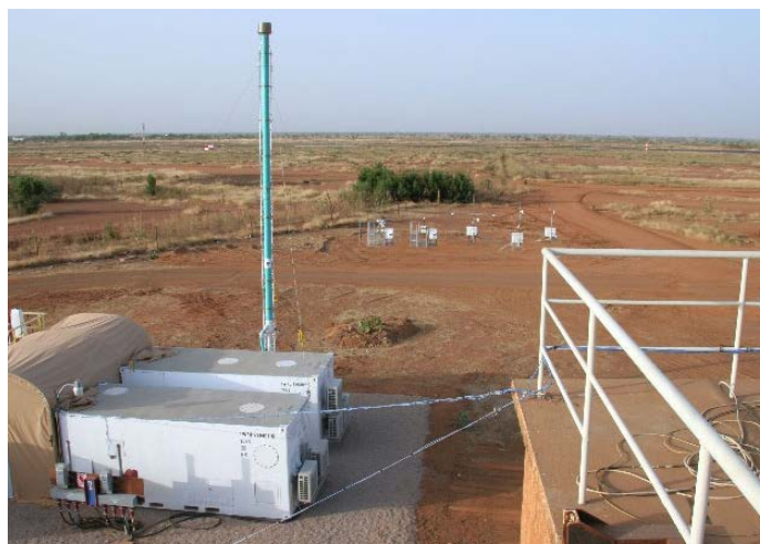
In 2006, AMF1 was deployed to Niamey, the capital of Niger, West Africa, for its second field campaign. Instruments, such as this aerosol stack, sampled absorbing aerosols from desert dust in the dry season and deep convective clouds and large column moisture loadings during the summer monsoon. There is still a need for additional observations of convective systems in arid and semi-arid environments.
