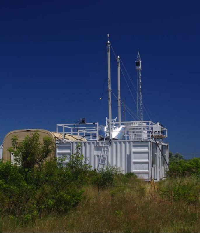
A collection of aerosol observing systems deployed with AMF1 to Cape Cod, Massachusetts, for 12 months starting in the summer of 2012. Smaller off-site campaigns that deploy subsets of the full AMF instrument suite could be beneficial in conducting studies with focused research questions.
