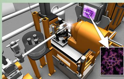
End-station concept of the macromolecular femtosecond crystallography instrument at the Linac Coherent Light Source. [Image courtesy SLAC National Accelerator Laboratory]
