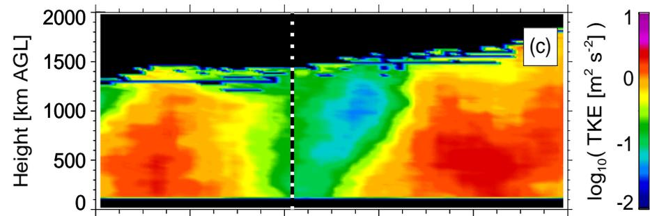
Response of the turbulent kinetic energy profile to the solar eclipse. Time of full eclipse indicated by dashed line.
