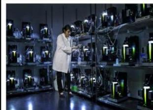
Programmable environmental photo-bioreactor array for laboratory simulation of algae growth in outdoor cultivation ponds.
