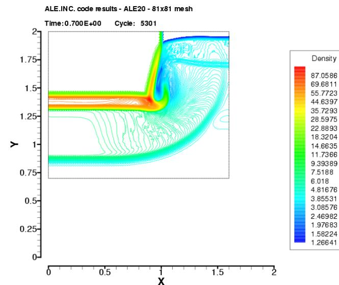
Interaction of Shock with heavy obstacle - ALE INC.(ubator)
