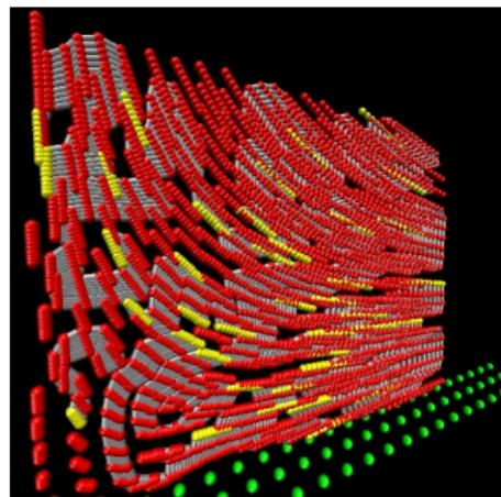
(LEFT) Uni-axial test: the molecules on right side are subjected to forces  $f$  and molecules to the left are constrained to zero displacement in  $x$ -direction.
