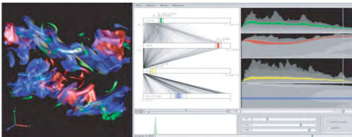
Figure 3. Interface for tri-space visual exploration of time-varying multivariate volume data [6]. From left to right, the spatial view, variable view, and temporal view of the data are given.
