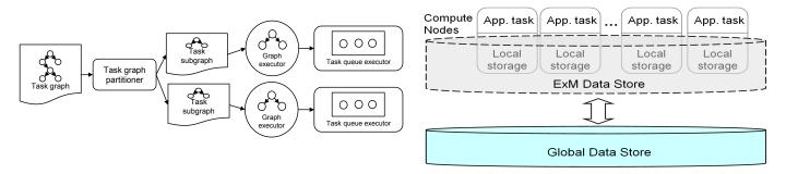
ExM complex-wide data storage – based on MosaStore – is embedded and distributed across nodes and RAM storage to provide a namespace and fast file data exchange.
