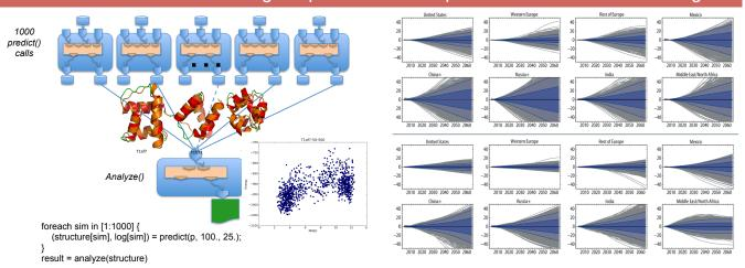
Simple Swift scripts (left) specify and execute 1,000 parallel tasks for protein structure prediction with Monte Carlo simulated annealing, and 5,000 models exploring uncertainty in consumer and industrial electricity usage (right).
