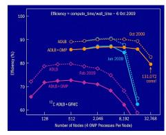
Traditional Master/Worker has a scaling bottleneck of worker ranks trying to access the shared queue managed by the master. ADLB scales to over 100K cores by making a shared queue accessible to all ranks without need to go through an arbiter process.
