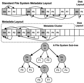
Figure 2: **Metadata clustering.** Each block corresponds to an i-node on disk. Shaded blocks labeled 'D' are directory i-nodes while non-shaded blocks labeled 'F' are file i-nodes. In the top disk layout, the indirection between directory and file i-nodes causes them to be scattered across the disk. The bottom disk layout shows how metadata clustering co-locates i-nodes for an entire sub-tree on disk to improve search performance.
