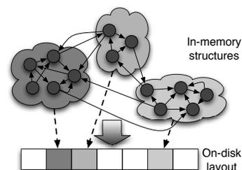
**Figure 1: Metadata clustering example.** Metadata clusters, partitions, shown in different shades, index different partitions of file system metadata. Each partition is stored sequentially on disk. The entire file system metadata index is composed of the set of all metadata clusters.
