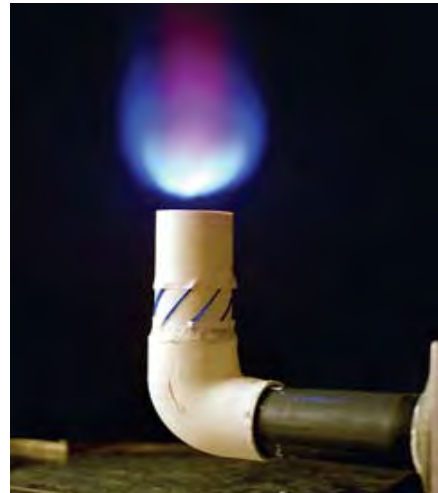
Figure 3. Low swirl burner prototype. The burner's novel flame stabilization mechanism allows it to operate at lean conditions with very low emissions (Photo courtesy of R. K. Cheng)
