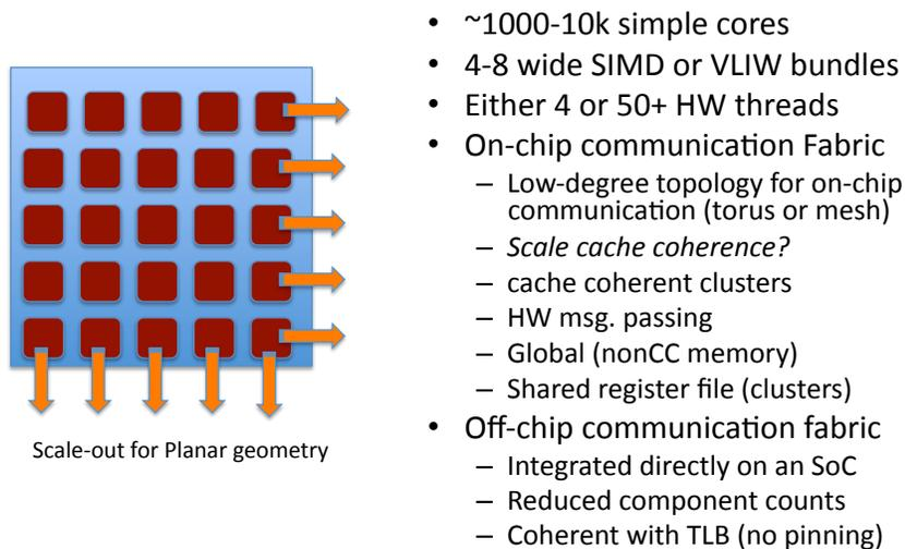
**Figure 3.6** Schematic of future node architecture. The number of functional units on the chip will need to scale out in a 2D planar geometry where locality of communication between the functional units will be increasingly important for efficient computation.
