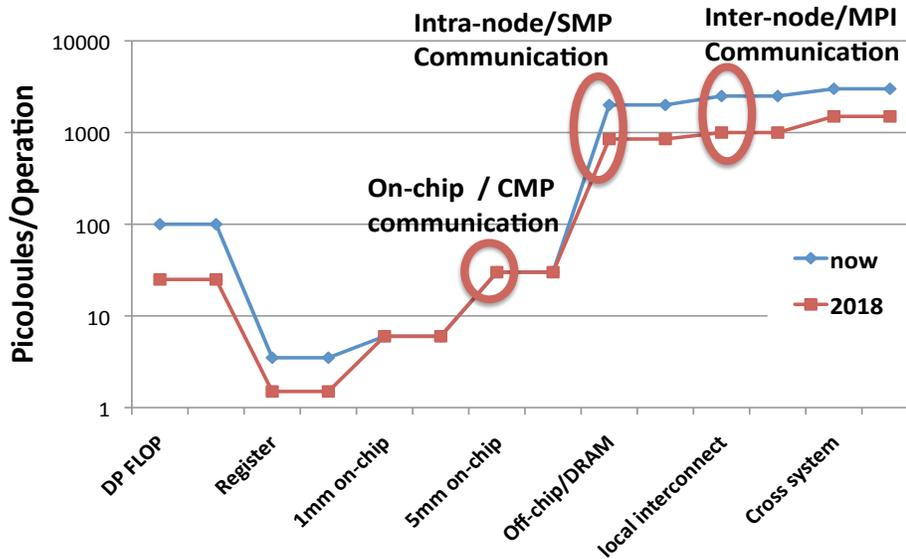
**Figure 3.1** Energy cost of data movement relative to the cost of a flop for now and for 2018 systems, without further investment. The biggest delta in energy cost is movement of data off-chip. Therefore, future programming-environments must support the ability of algorithms and applications to exploit locality, which will, in turn, be necessary to achieve performance and energy efficiency.
