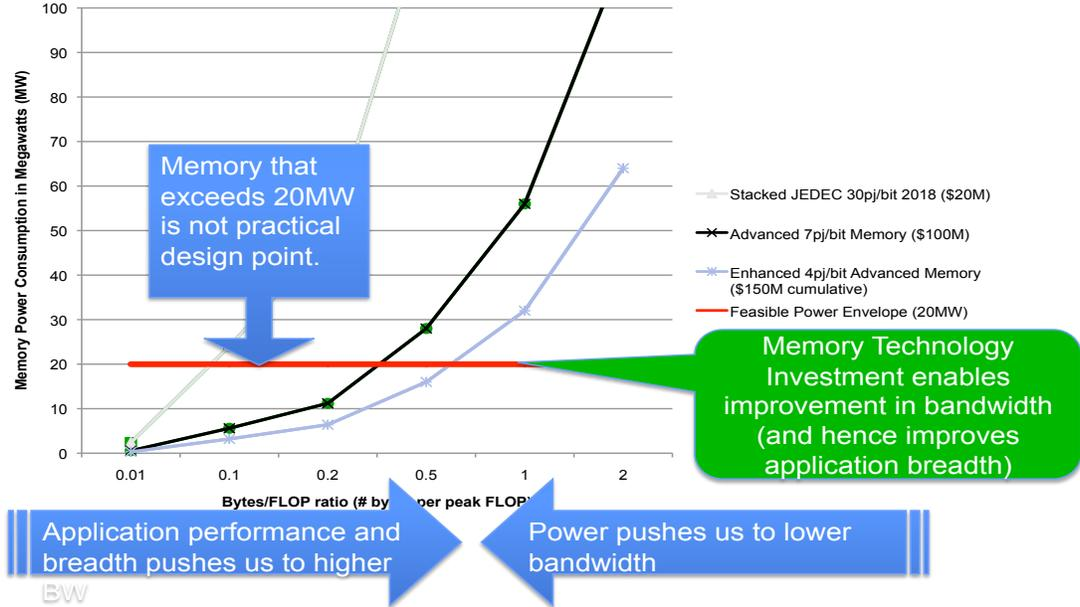
**Figure 3.3** This figure illustrates the trade-offs between memory power consumption and the desire for a more broadly applicable exascale system design under different assumptions about investment in advanced memory technology.
