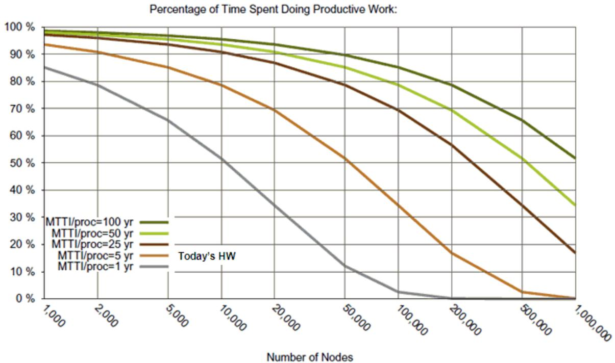
**Figure 1.1** As the number of nodes increases, the time between faults decreases; hence, the frequency of checkpointing must also increase. The graph shows how the time spent doing checkpointing decreases the percentage of time doing productive work (assuming different hardware resilience targets).
