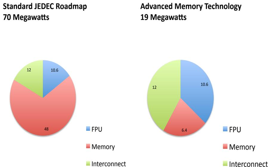
**Figure 3.2.** If we follow standard JEDEC memory technology roadmaps, the power consumption of a feasible exascale system design (using 0.2 bytes/flop memory bandwidth balance) will be >70 MW due to memory power consumption, which is an impractical design point. Keeping memory power under control will either require substantial investments in more efficient memory interface protocols, or substantial compromises on memory bandwidth and floating point performance (< 0.02 bytes/flop).
