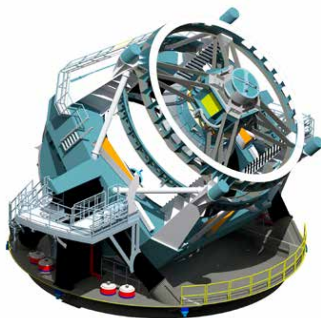
An artist's rendering of the proposed Large Synoptic Survey Telescope. The 8.4-meter LSST will use a special three-mirror design, creating an exceptionally wide field of view and will have the ability to survey the entire sky in only three nights. (Courtesy: LSST Corporation)
