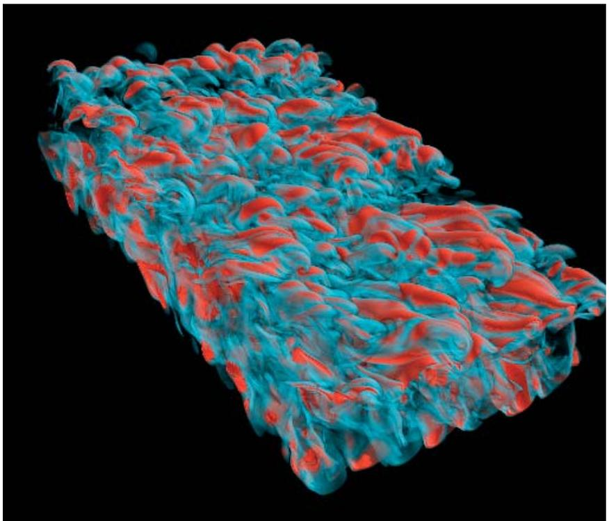
**FIGURE 1.** A simulated planar jet flame, colored by the rate of molecular mixing (scalar dissipation rate), which is critical for determining the interaction between reaction and diffusion in a flame. The image shows that high scalar dissipation regions exist in thin, highly intermittent structures aligned with principal strain directions. (Visualization created using an application written by Hongfeng Yu and Kwan-Liu Ma, UC Davis.)
