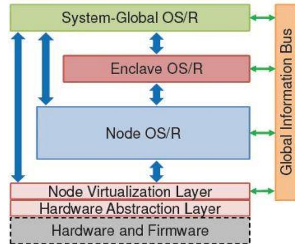
Schematic representation of the main components of the Hobbes architecture and their interactions via APIs (vertical arrows) and data exchange (horizontal arrows).
