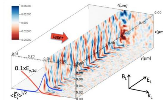
Field fluctuations [ $E_y - E_y, 1d$ ] due to plasma waves in a highly resolved 3D PIC simulation, shown near the target surface at  $z = 0.25 \mu\text{m}$ . Laser is incident from  $z = 0$ .
