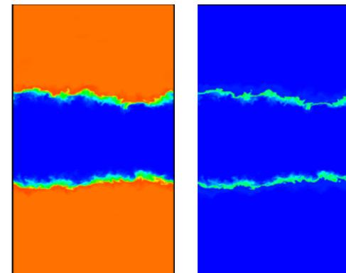
*Snapshot images from simulation of periodic turbulent reacting jet (flow left to right). Transport part of the Navier-Stokes equations solved with CPUs and chemistry parts solved with GPUs.*
