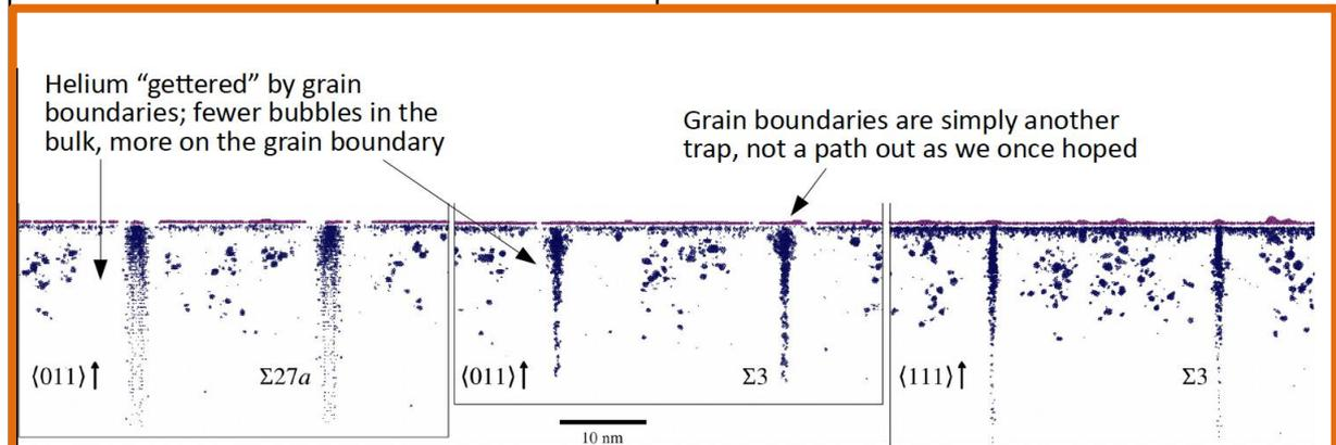
MD simulations showing helium (blue spheres) located below tungsten surfaces with grain boundaries that intersect the surface, as a function of surface orientation. Tungsten atoms displaced to the surface by the clustering phenomena are shown as purple spheres.
