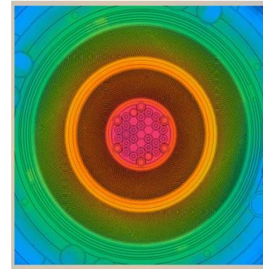
*Neutron flux in a detailed simulation of the HFIR core*
