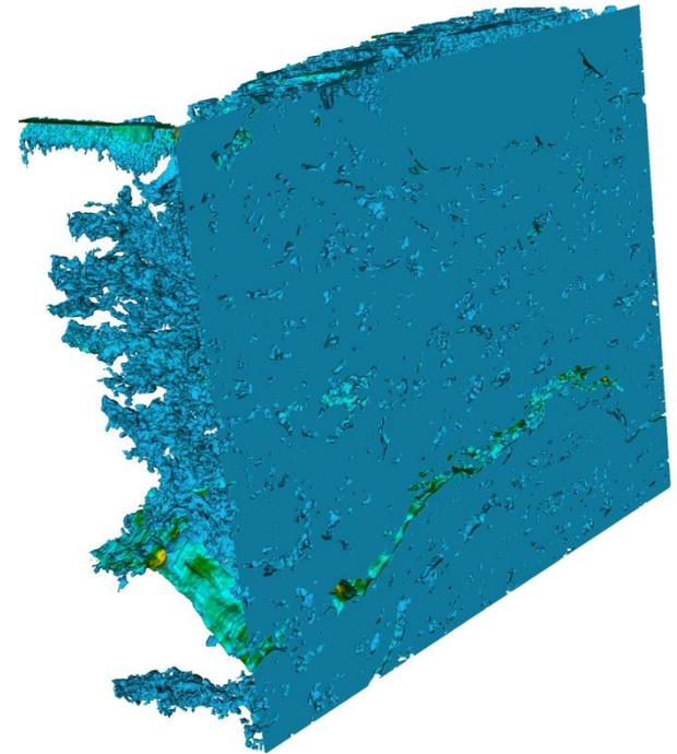
Simulation of resolved flow in Marcellus shale. Projected surface plot of velocity shown. Simulation performed on 60,000 cores NERSC Hopper. Data is based upon FIB-SEM imagery obtained by Lisa Chan at Tescan USA and processed by Terry Ligocki (LBNL), courtesy of Tim Kneafsey (LBNL)
