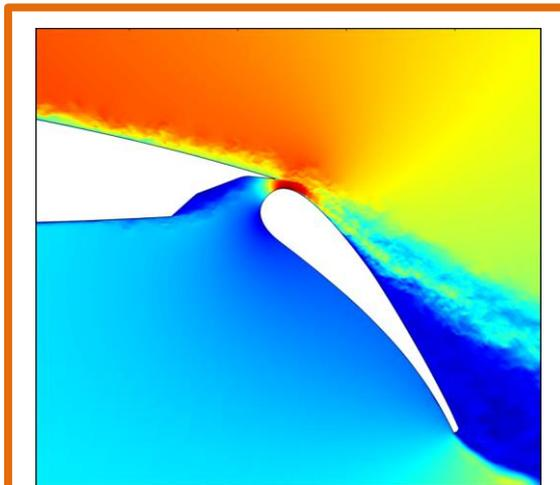
Streamwise velocity contours near multi-element airfoil flap.
