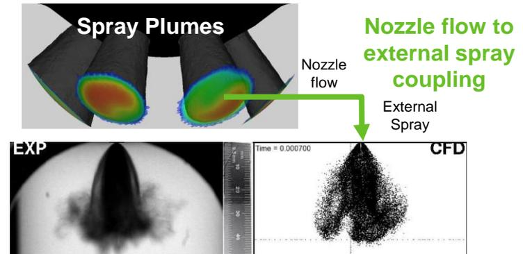
Internal nozzle flow computations are used to initialize external spray calculations. The procedure is validated against experiments.
