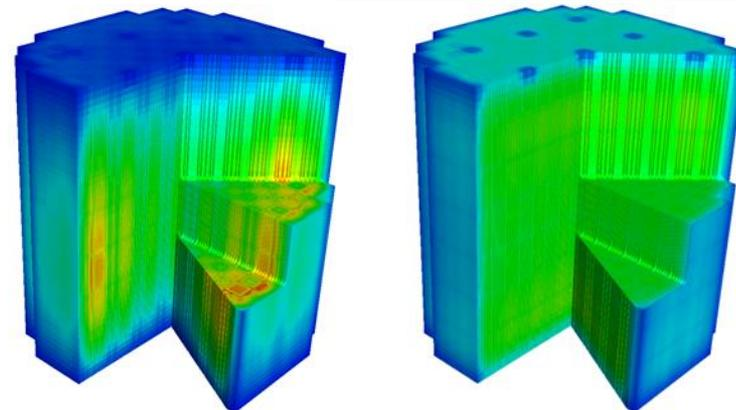
*The beginning (left) and end (right) from a simulation of 3D pin power distribution at the Watts Bar nuclear power plant.*
