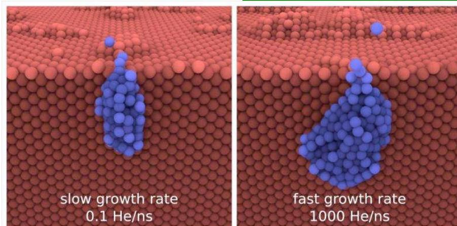
ParRep simulation of the tungsten surface morphology for helium bubbles growing inside a fusion reactor divertor.
