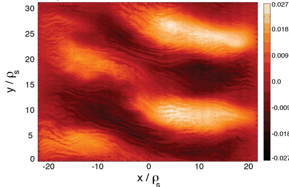
Snapshot of predicted midplane fluctuations in the Alcator C-Mod tokamak
