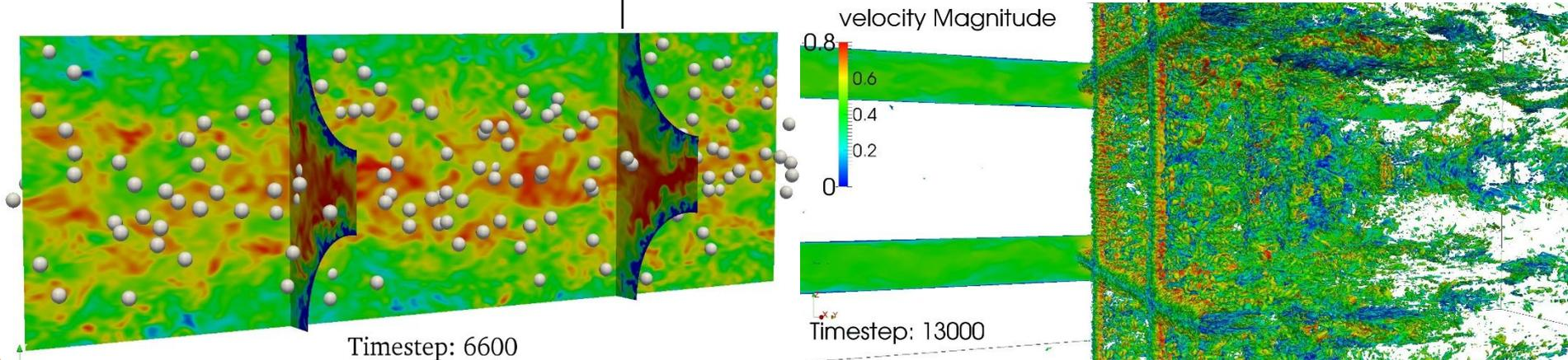
Bubbly flow simulation in a nuclear reactor subchannel (1B elements with 260 bubbles, left) and reactor coolant flow through PWR core with fully resolved mixing vanes and spacer grids (2B elements at 1/10 reactor flow, right)
