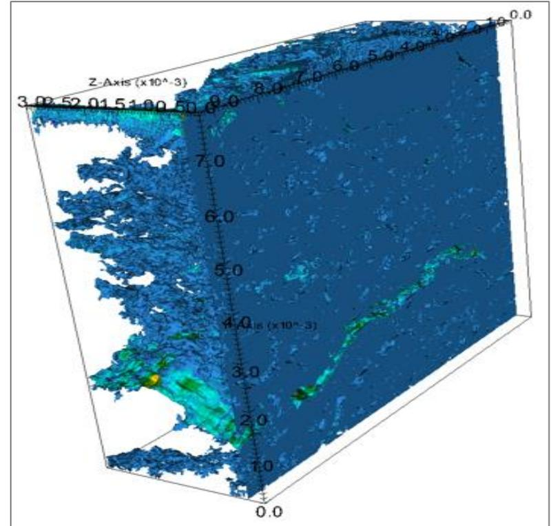
**Simulation** of flow in fractured Marcellus shale using 60,000 cores of Hopper. Fluid velocity shown with 48-nm resolution. Sample courtesy of Tim Kneafsey (LBNL), imaged at Tescan USA.
