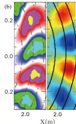
Contour plot of relative electron temperature on a poloidal plane from a GTC simulation. The images are a comparison of structure from the simulation (left) and from the DIII-D experiment (right) in the ECEI window. The red color represents positive perturbations and the blue color represents negative perturbations. *Image credit: Wang, et al. PRL 111, 145003 (2013)*
