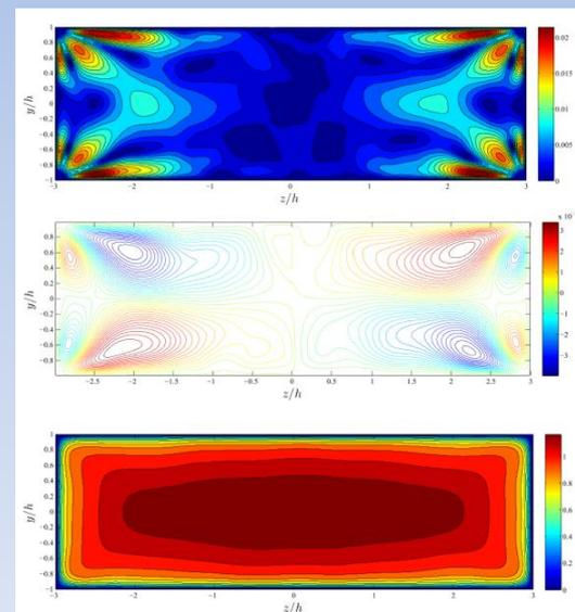
(Right) Duct aspect ratio (width/length) 3 in-plane velocity, streamlines and streamwise velocity. Friction actually increases in this case over square duct cross section due to 3-dimensional effects difficult to measure in experiments.
