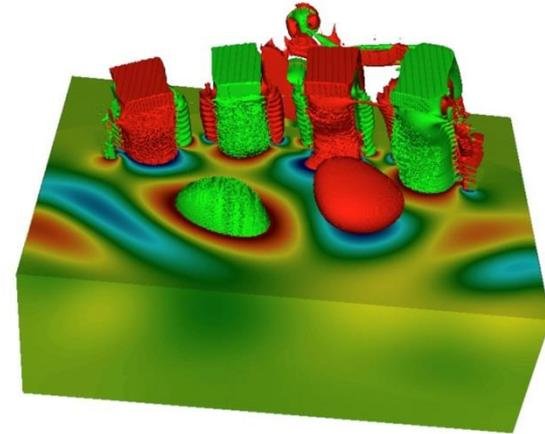
Simulation of the Alcator C-Mod Field Aligned Antenna in pi-mode. The left plot shows fast wave propagation from the antenna for high-edge density. If slow waves are present, their field amplitudes can be high and can contribute to both the amplitude of the radio frequency sheath voltage and to parasitic power losses in the edge plasma.
