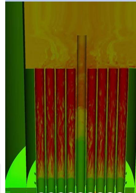
(Right) Temperature distribution in the MASLWR core computed using Nek5000 (frozen velocity)
