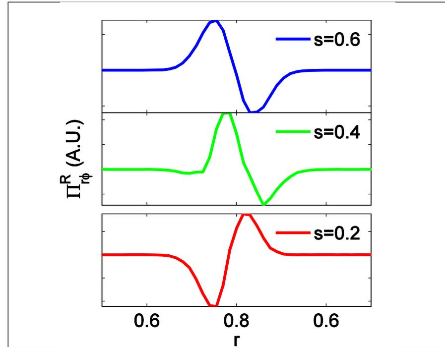
As magnetic shear ( $s$ ) decreases from 0.6 to 0.2, a specific momentum flux ( $\Pi_{T\phi}^R$ ) that drives intrinsic rotation changes orientation, indicating the intrinsic torque reversal.
