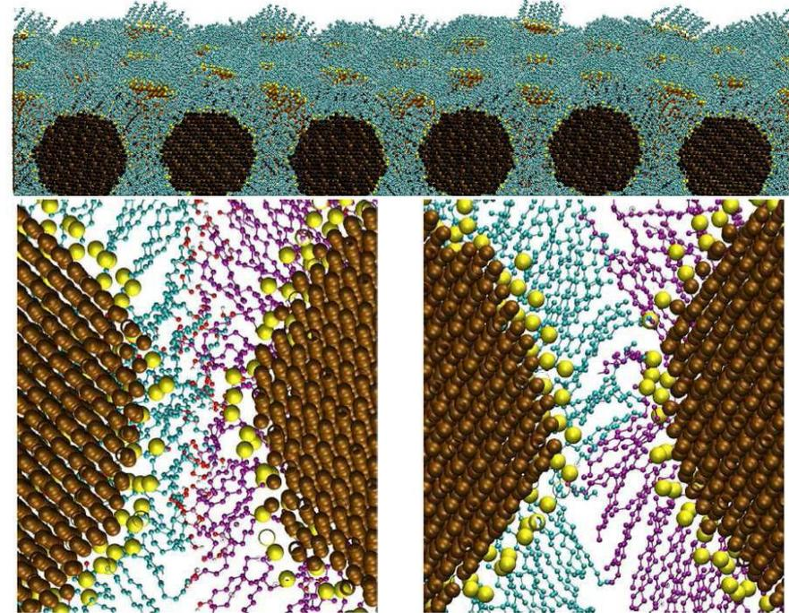
Top: angled side view of  $\text{CH}_3$ -terminated dry membrane prior to deformation. H atoms are represented in white, C: cyan, Au: brown, and S: yellow. Bottom: close-up of COOH terminated (left) and  $\text{CH}_3$ -terminated (right) nanoparticles. Hydrogen atoms have been omitted except in the COOH end group. C atoms on the left NP are colored cyan while those on the right are colored purple.
