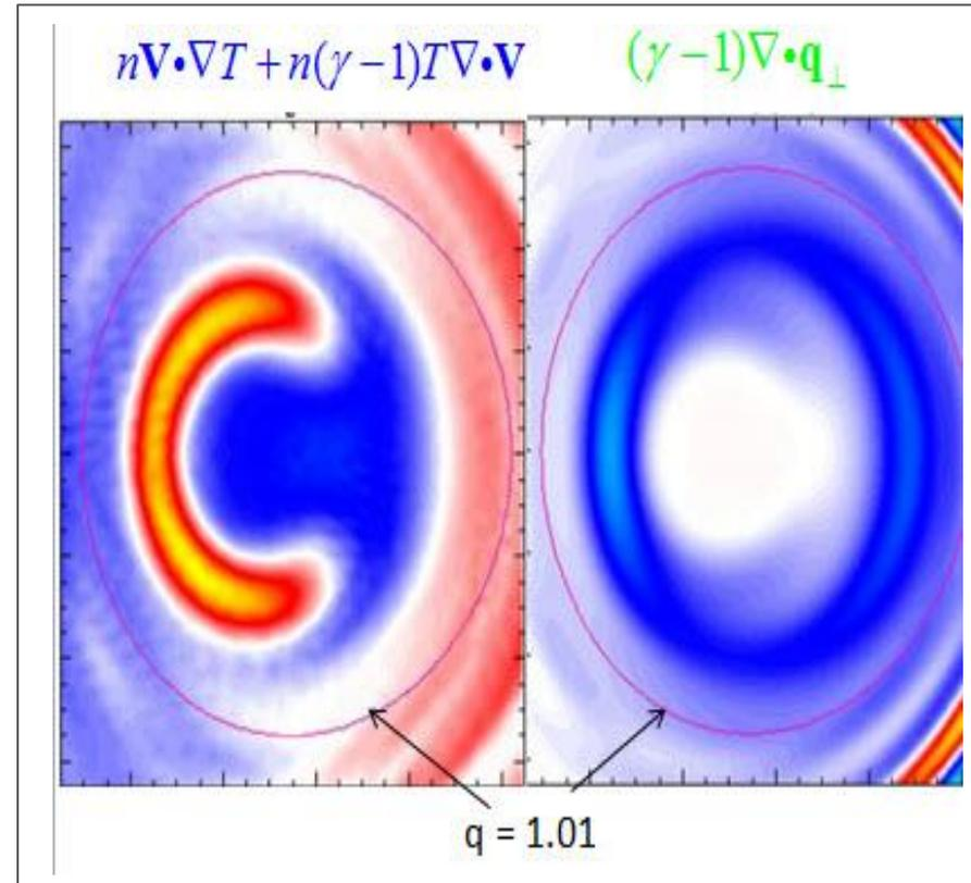
**Terms in the energy balance** for the temperature equation at one toroidal location in the plasma core for stationary state. Left frame shows terms driven by velocity. Right shows normal loss terms.
