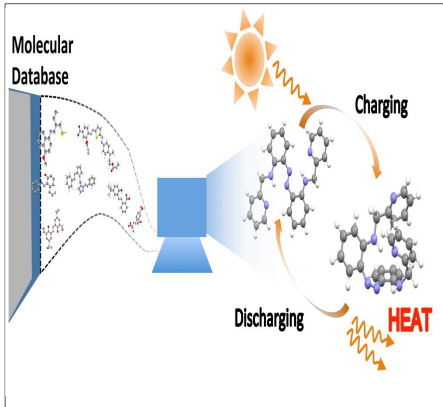
**Schematic** showing the workflow involved in identifying new materials that store the energy of sunlight by changing the organization of atoms in a molecule, later to reorganize back to the original structure and release the energy as heat.
