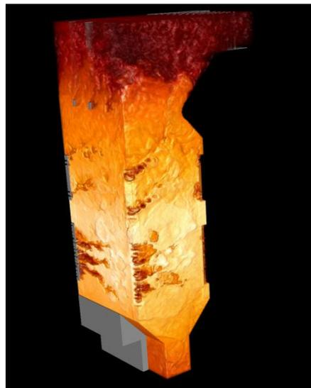
*Boiler Simulation Facility temperature field demonstrating the gas temperature field from a typical large eddy simulation.*
