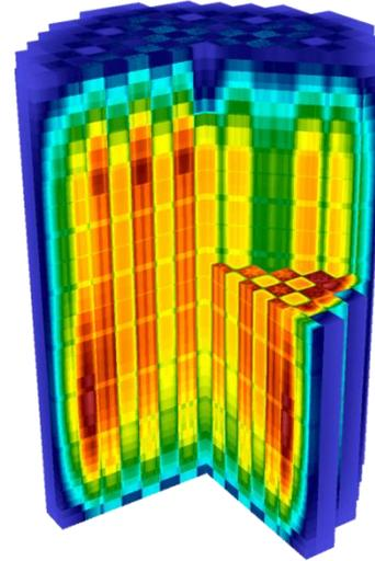
Center for the Advanced Simulation of Lightwater Reactors (CASL) investigators successfully performed full core physics power-up simulations of the Westinghouse AP1000 pressurized water reactor core using their Virtual Environment for Reactor Application code that has been designed on Titan architecture.
