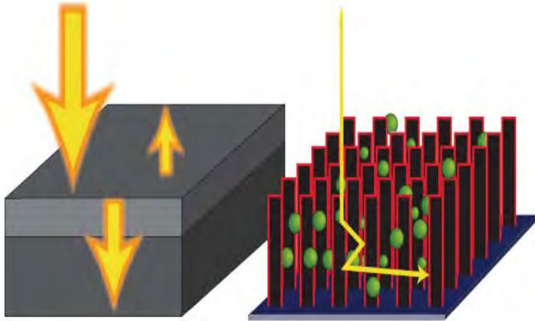
**Figure 1** | Solar-cell light management. **a**, Conventional thin-film solar cells where incident light gets partially reflected. **b**, In the microwire arrays, Al<sub>2</sub>O<sub>3</sub> nanoparticles (shown in green) reflect incident light and redirect it towards the micropillars.
