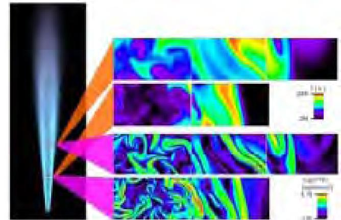
Top: Direct numerical simulation of a CO/H<sub>2</sub> slot flame
