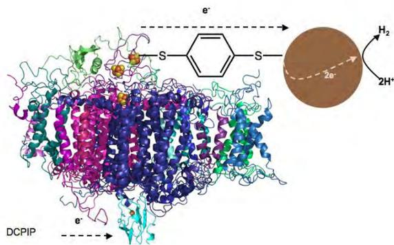
PS-I covalently attached to nanoparticle catalysts via a molecular wire yields 75% of plant electron transfer rates resulting in photo-generated hydrogen at ~1700 X current benchmarks
