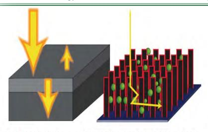
Figure 1 | Solar-cell light management. **a**, Conventional thin-film solar cells where incident light gets partially reflected. **b**, In the microwire arrays, Al<sub>2</sub>O<sub>3</sub> nanoparticles (shown in green) reflect incident light and redirect it towards the micropillars.
