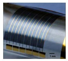
Flexible solar cells with efficiencies of ~12% and silicon thicknesses of 15 µm
