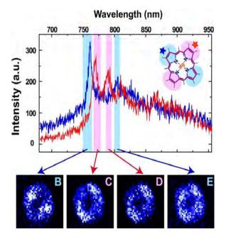
Scanning tunneling microscope images produced while monitoring the emission spectrum of a single molecule show, with atomic resolution, different spectra emitted from different locations on the molecule, giving an unprecedented atomic-level view of the coupling of electronic and vibrational motion. (Wilson Ho, UC Irvine)
