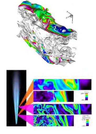
Top: Direct numerical simulation of a CO/H2 slot flame Bottom: Imaging of a model flame jet flame
