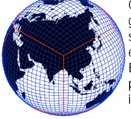
Cubed-sphere grid of CAM spectral element model. Fach cube panel is divided into elements.
