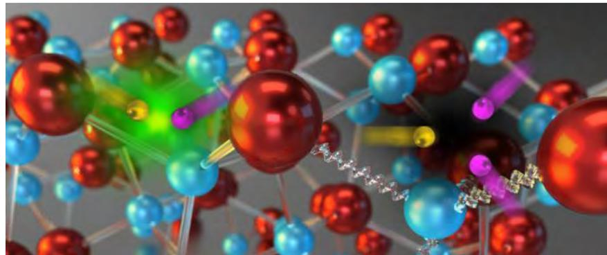
Schematic of an LED crystal. At left, an electron and electron hole recombine and release light. In Auger recombination (right) the electron and hole combine with a third carrier, releasing no photon. The energy loss is also assisted by indirect processes, vibrations in the crystal lattice shown as squiggles.
